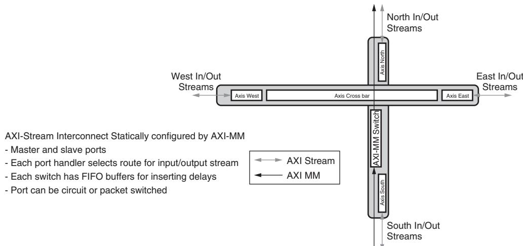
**Figure 6: AI Engine Array AXI-MM and AXI-Stream Interconnect**
