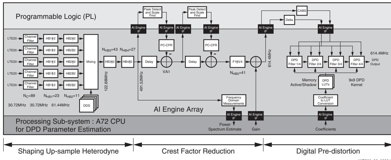
Figure 9: Block Diagram: 100MHz 5-Channel LTE20 Wireless Solution with DSP
