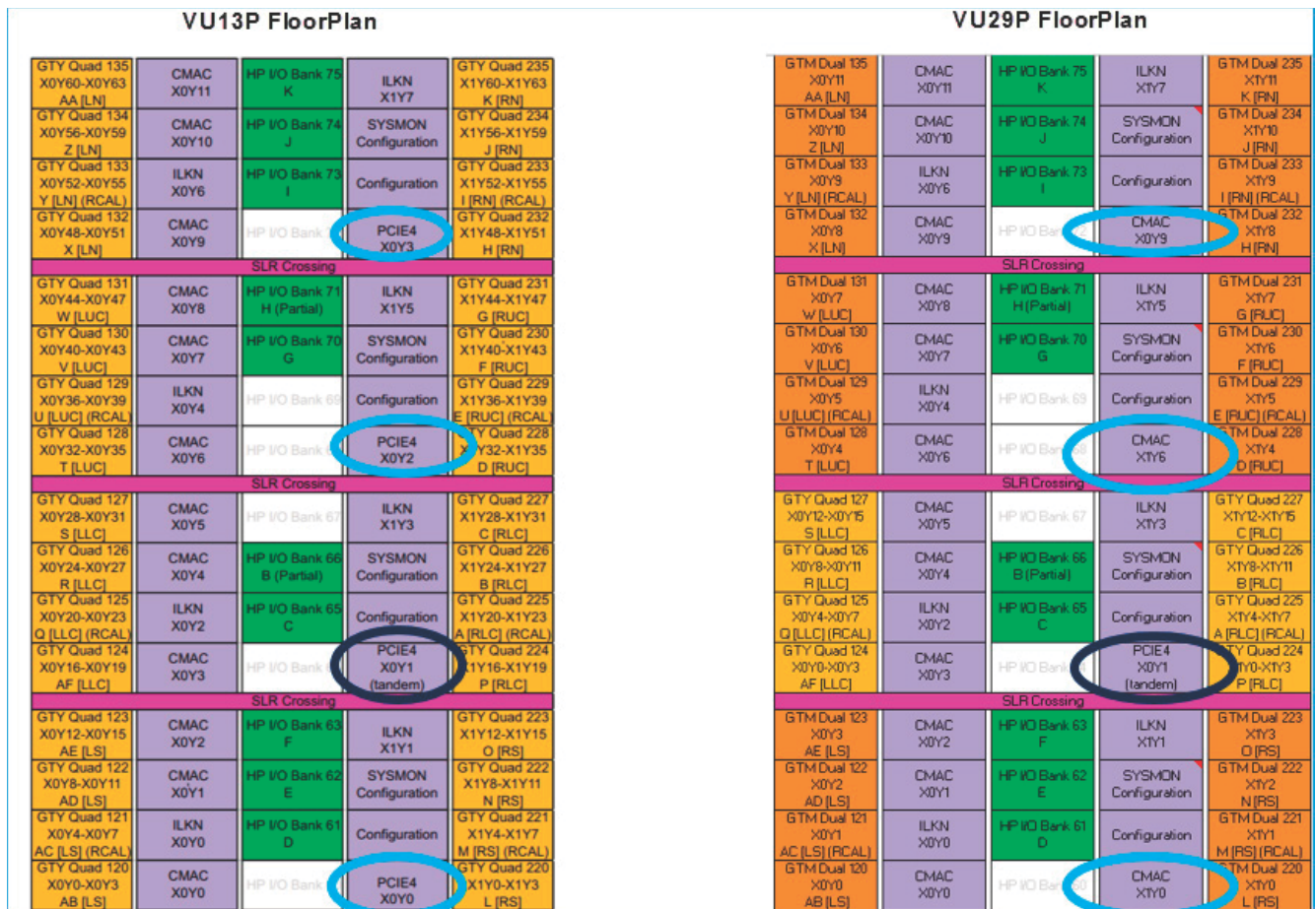
Figure 9-5: VU13P Floorplan with PCIe/GTY versus VU29P Floorplan with CMAC/GTM
