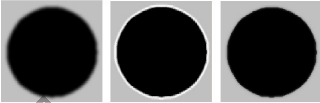
Figure 3-5: Original Defocused Image, Edge Enhanced Image, without and with Anti-Halo
