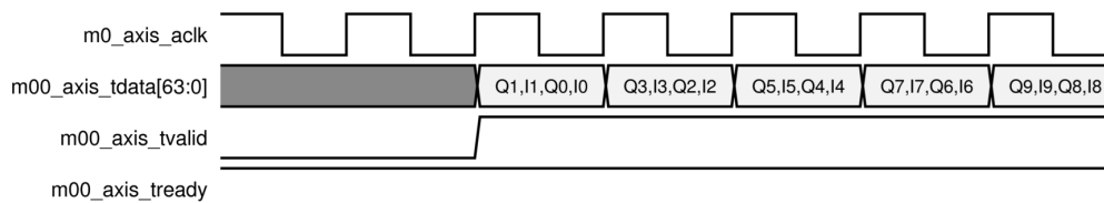
Figure 130: Single RF-ADC Output
