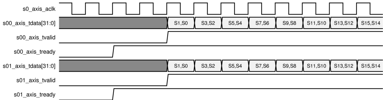
Figure 131: Two RF-DACs with Real Data on Separate Interfaces at 250 MHz
