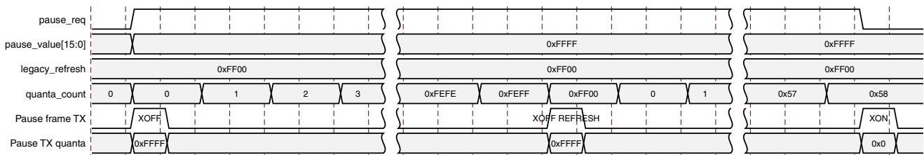
Figure 3-34: XON/XOFF Frame Transmission
