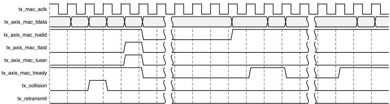
Figure 3-28: Collision Handling – No Frame Retransmission Required
