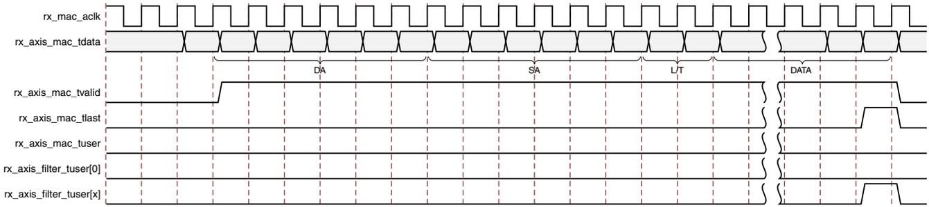
Figure 3-36: Received Frame with a Match on Filter 0
