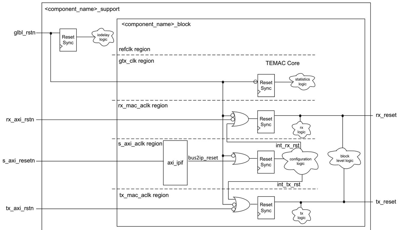
Figure 3-8: Reset Architecture
