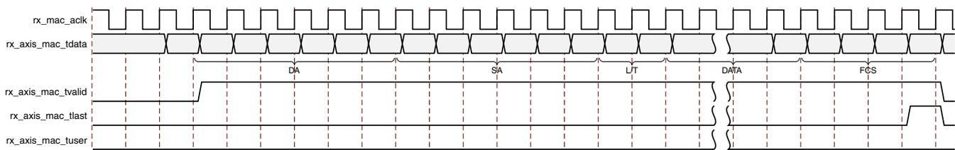
Figure 3-17: Frame Reception with In-Band FCS Field
