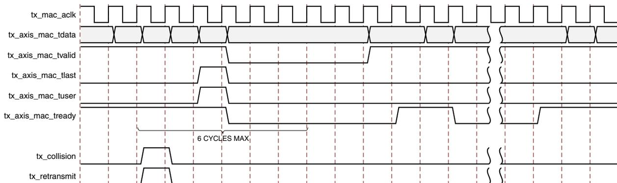
Figure 3-27: Collision Handling – Frame Retransmission Required
