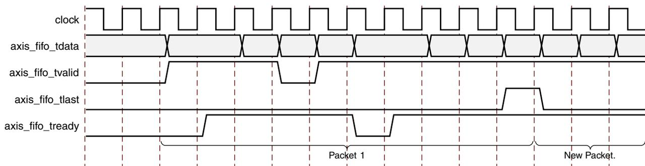
Figure 8-2: Frame Transfer across AXI4-Stream Interface
