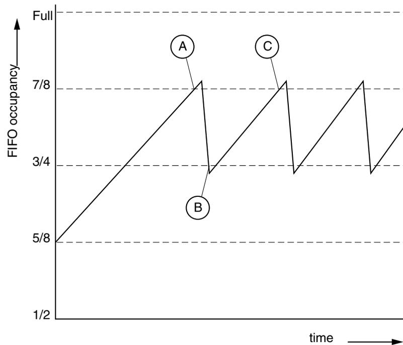
Figure 3-34: **Flow Control Implementation Triggered from FIFO Occupancy**
