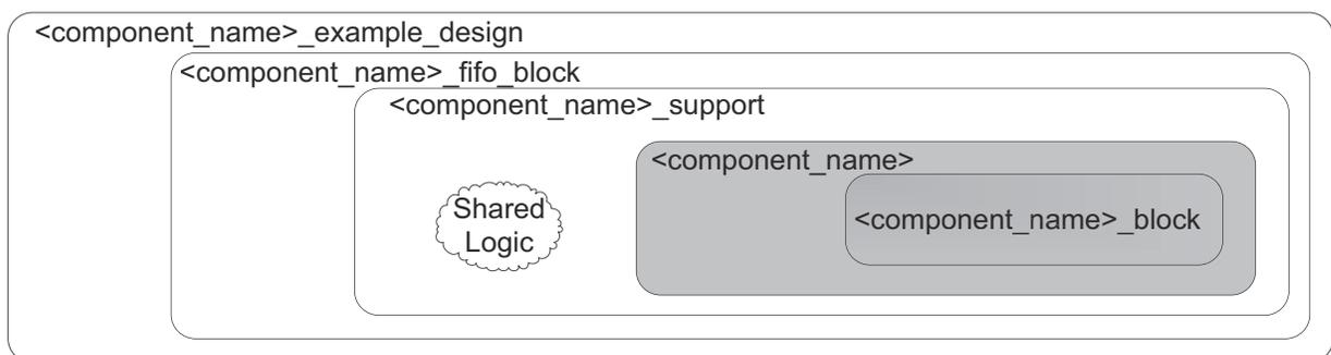
Figure 3-3: Shared Logic Included in Example Design
