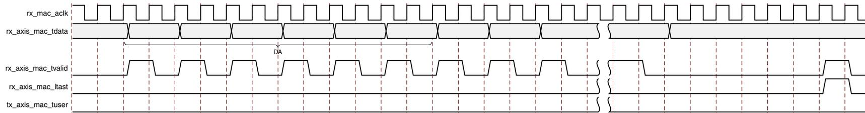
Figure 3-13: Normal Frame Reception at 10/100 Mb/s
