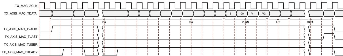
Figure 3-26: Transmission of a VLAN Tagged Frame
