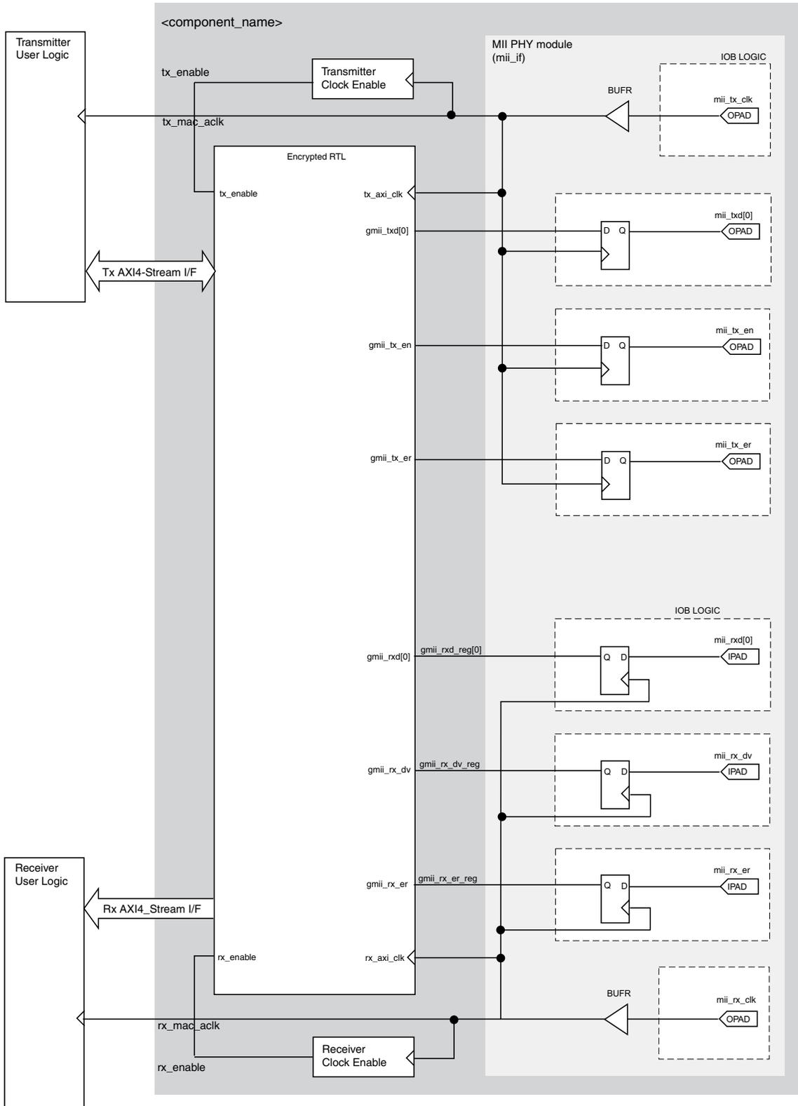
Figure 3-55: MII Transmitter, Receiver and Clock Logic For All Devices
