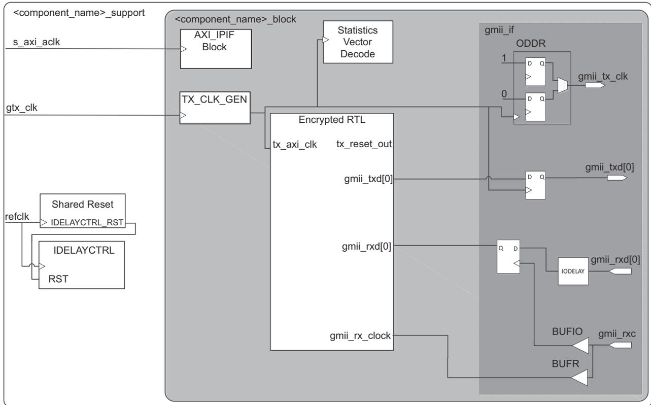
Figure 3-6: GMII Logic for 7 Series Devices
