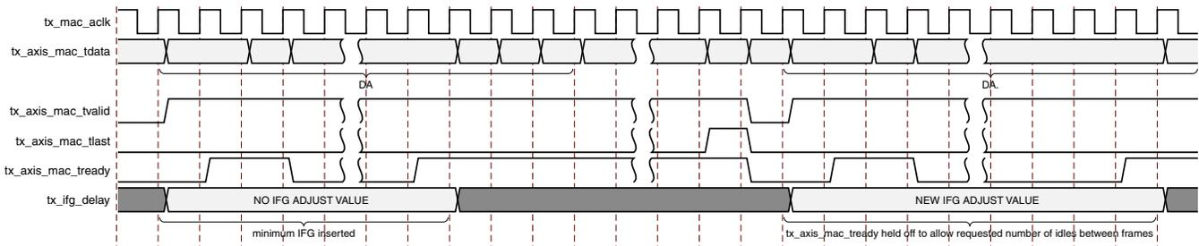
Figure 3-29: Interframe Gap Adjustment
