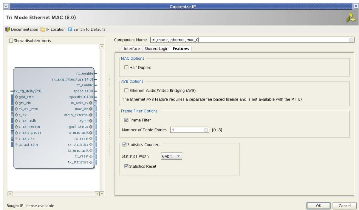
Figure 4-2: Vivado Customize IP IDE – Features Tab
