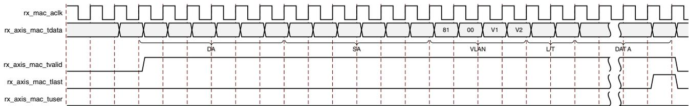
Figure 3-18: Reception of a VLAN Tagged Frame
