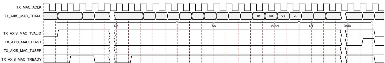
Figure 3-21: Transmission of a VLAN Tagged Frame
