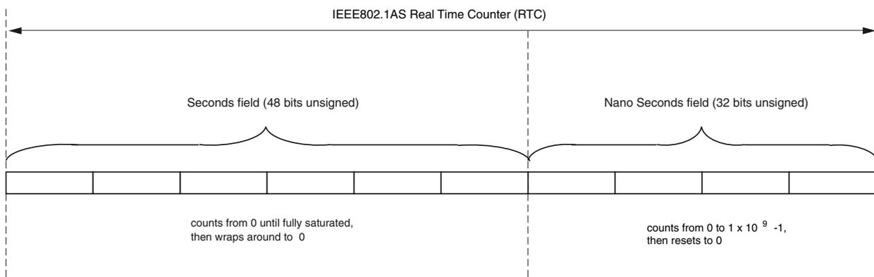
Figure 3-38: Real-Time Clock (RTC)
