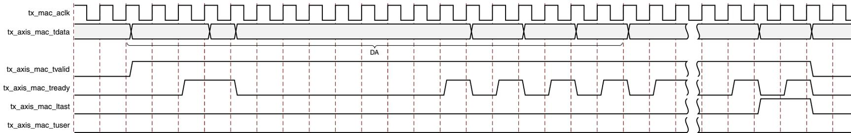
Figure 3-16: Normal Frame Transmission at 100 Mb/s Across User Interface (MII/GMII)
