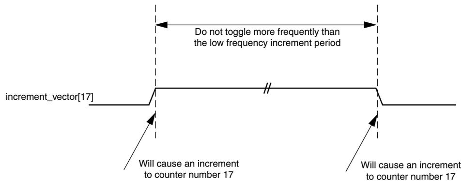
**Figure 3-30: Increment Vector Timing Diagram**
