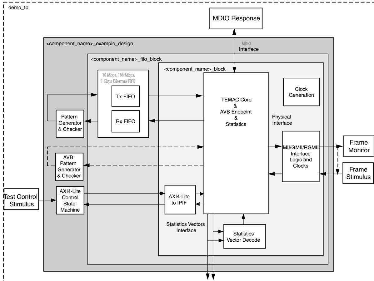
Figure 6-6: Demonstration Test Bench
