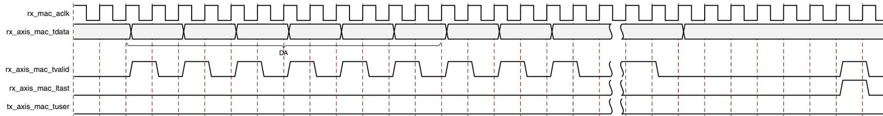
Figure 3-8: Normal Frame Reception at 10/100 Mb/s
