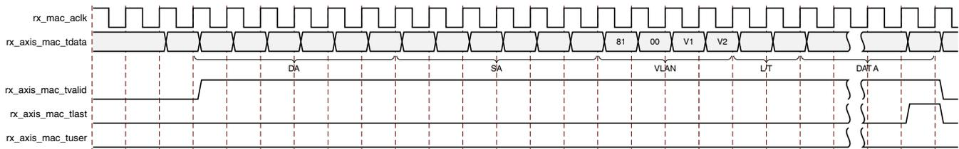
Figure 3-13: Reception of a VLAN Tagged Frame
