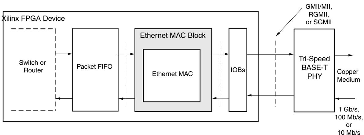
Figure 1-3: Typical Application: Ethernet Switch or Router
