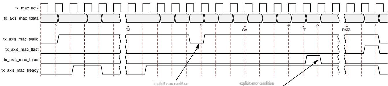
Figure 3-19: Frame Transmission with Underrun
