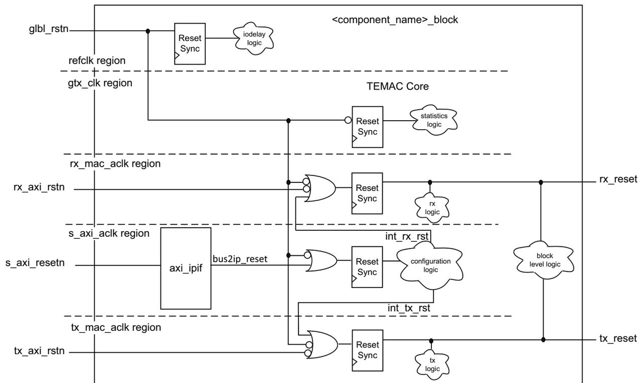
Figure 3-3: Reset Architecture
