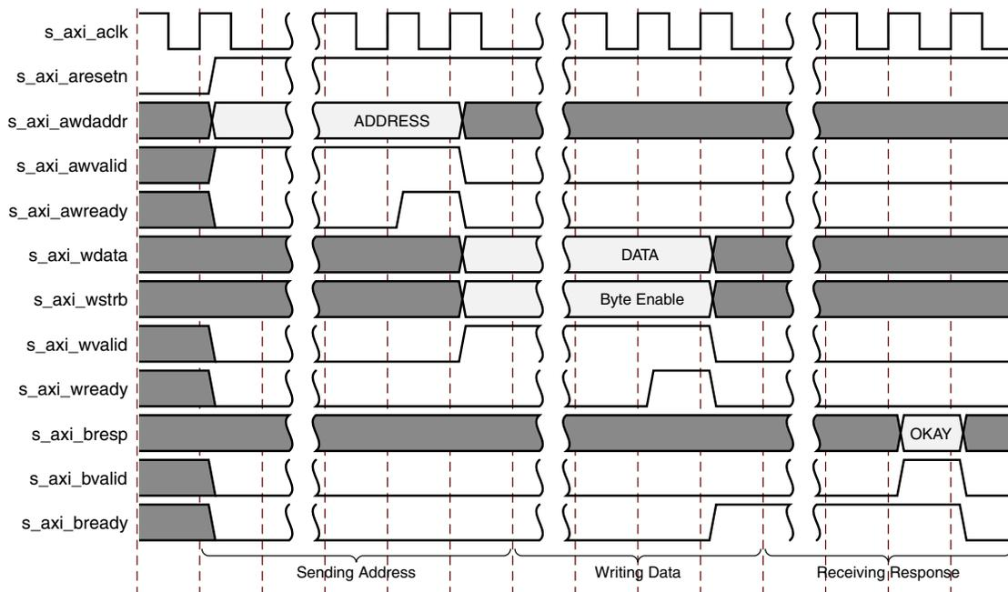
Figure 3-43: Management Register Write Timing
