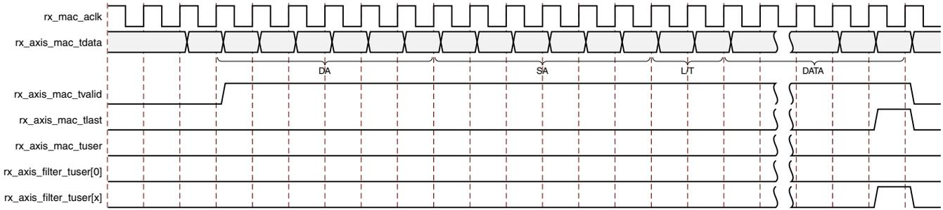
Figure 3-31: Received Frame with a Match on Filter 0
