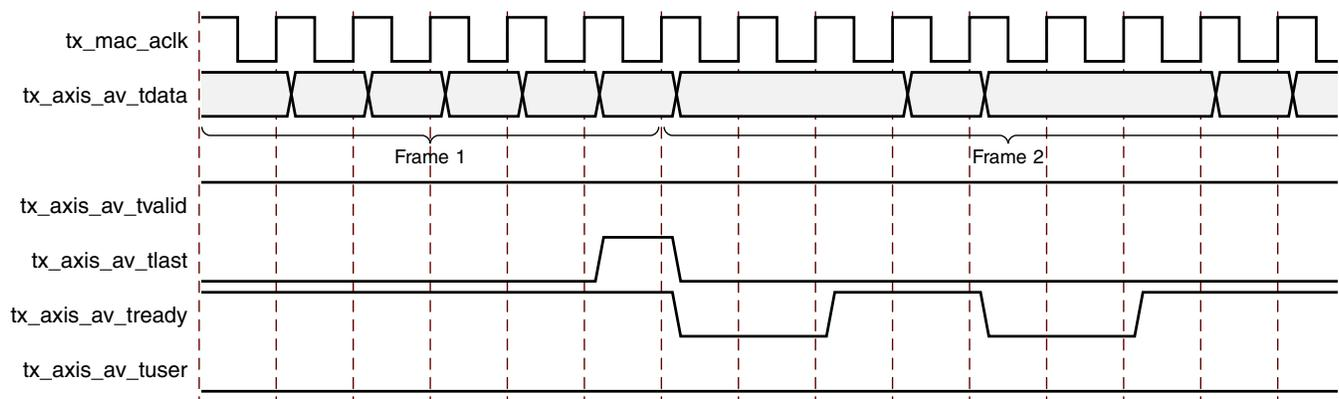
Figure 3-36: TX AV Traffic Timing
