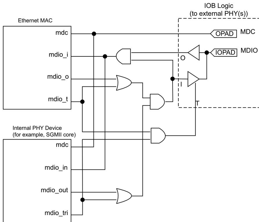
Figure 3-49: Internal and External MDIO Interfaces
