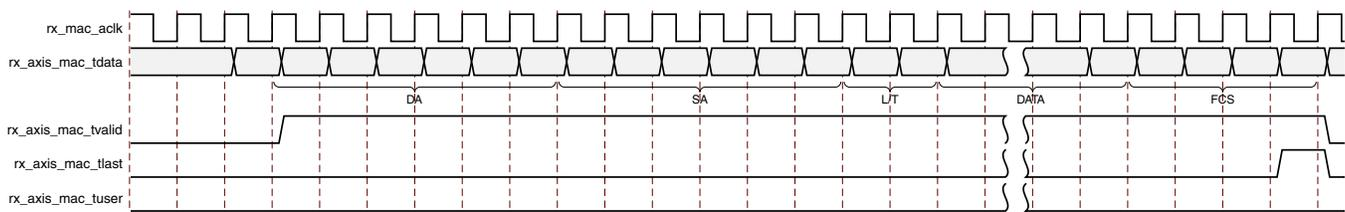
Figure 3-12: Frame Reception with In-Band FCS Field
