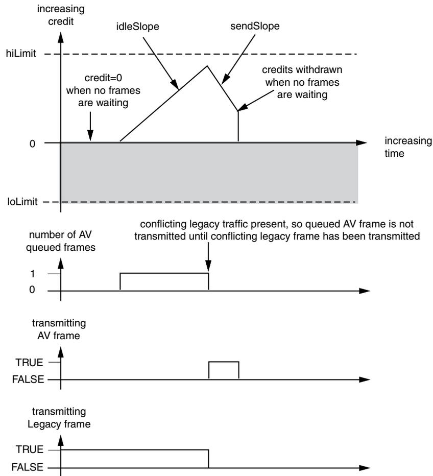
Figure 3-37: Credit-Based Shaper Operation
