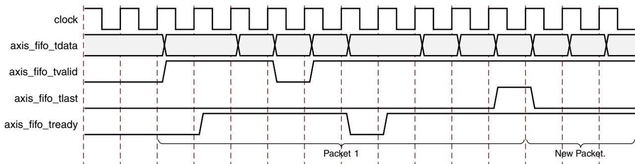
Figure 6-2: Frame Transfer across AXI4-Stream Interface
