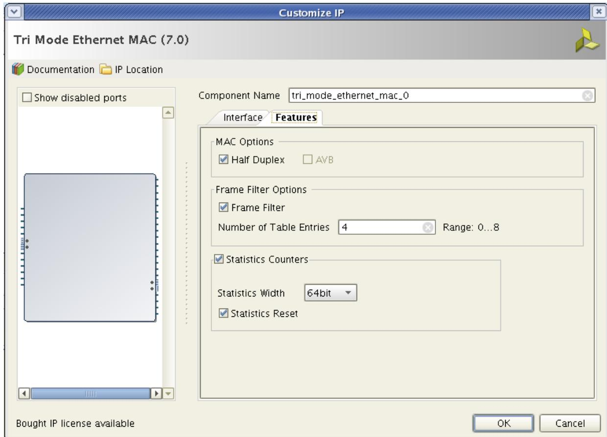
Figure 4-2: Vivado Customize IP IDE – Features Tab
