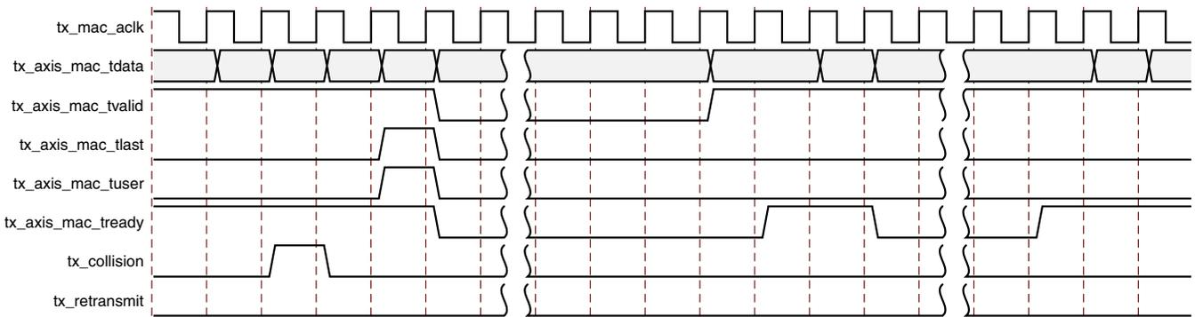
Figure 3-23: Collision Handling – No Frame Retransmission Required
