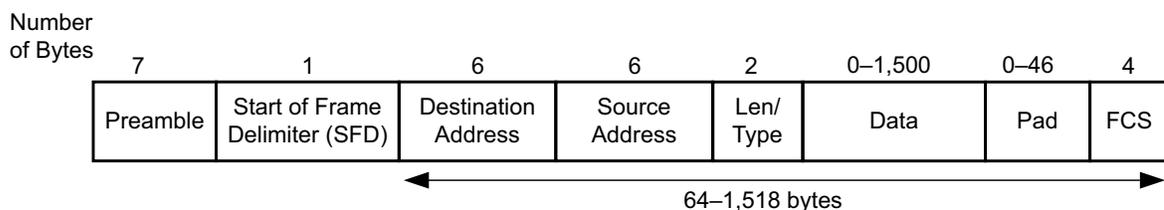
Figure 3-5: Standard Ethernet Frame Format
