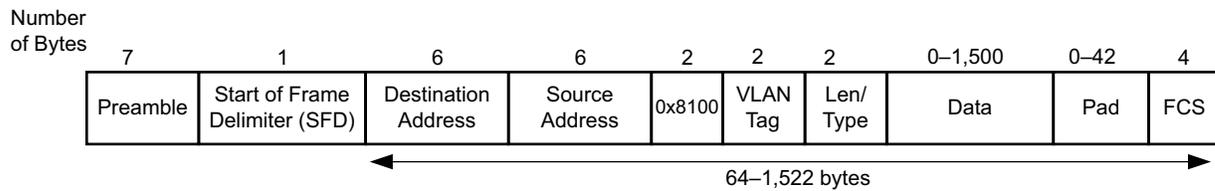
Figure 3-6: Ethernet VLAN Frame Format
