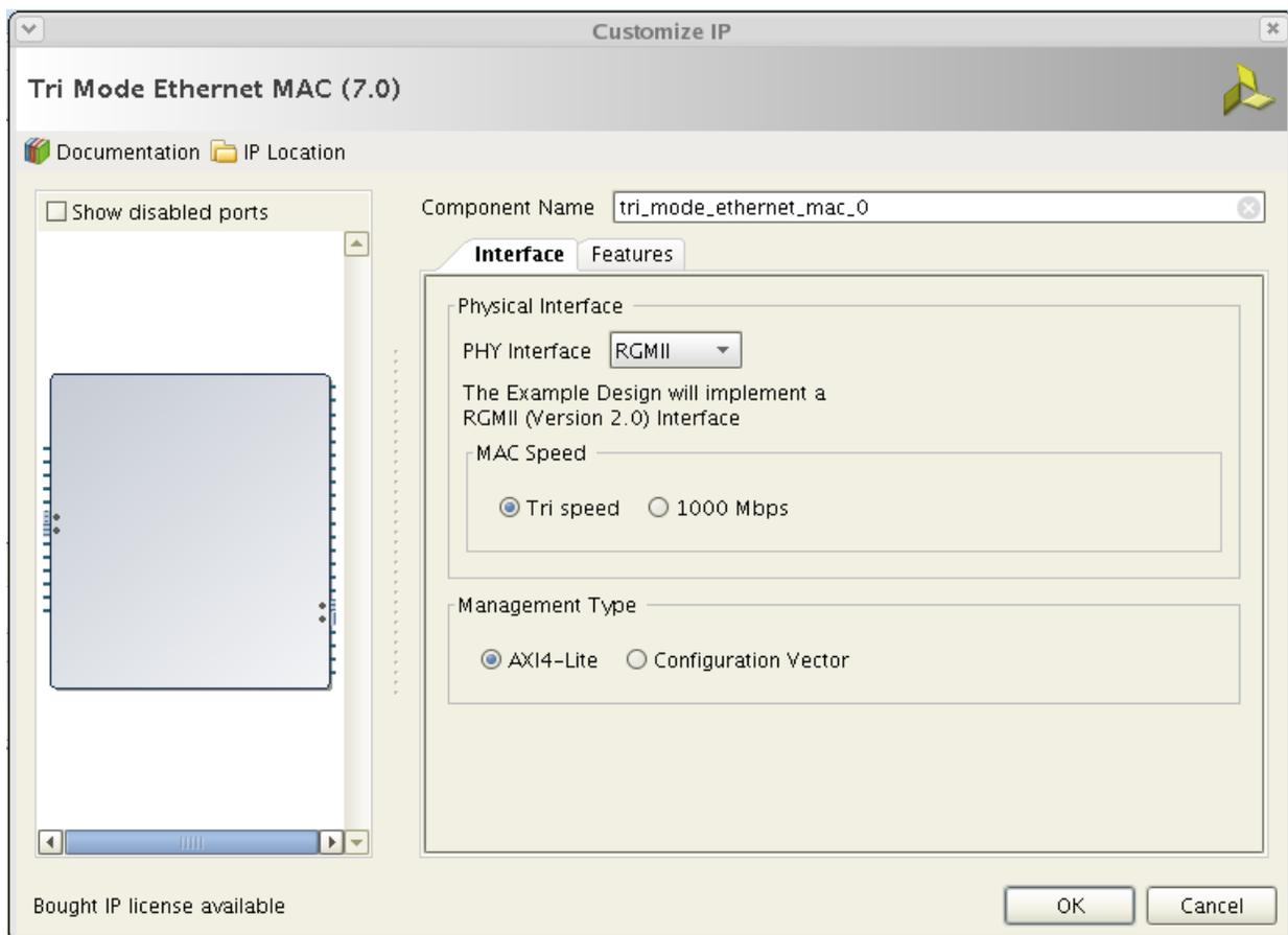
Figure 4-1: Vivado Customize IP IDE – Interface Tab
