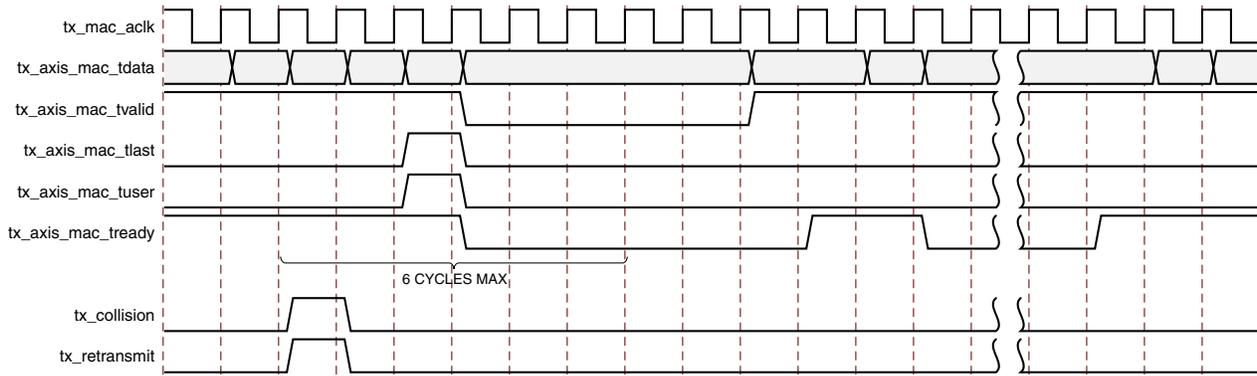
Figure 3-22: Collision Handling – Frame Retransmission Required
