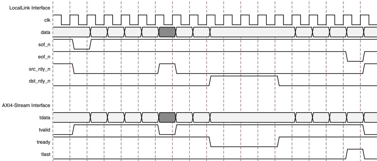
Figure C-11: LocalLink versus AXI4-Stream
