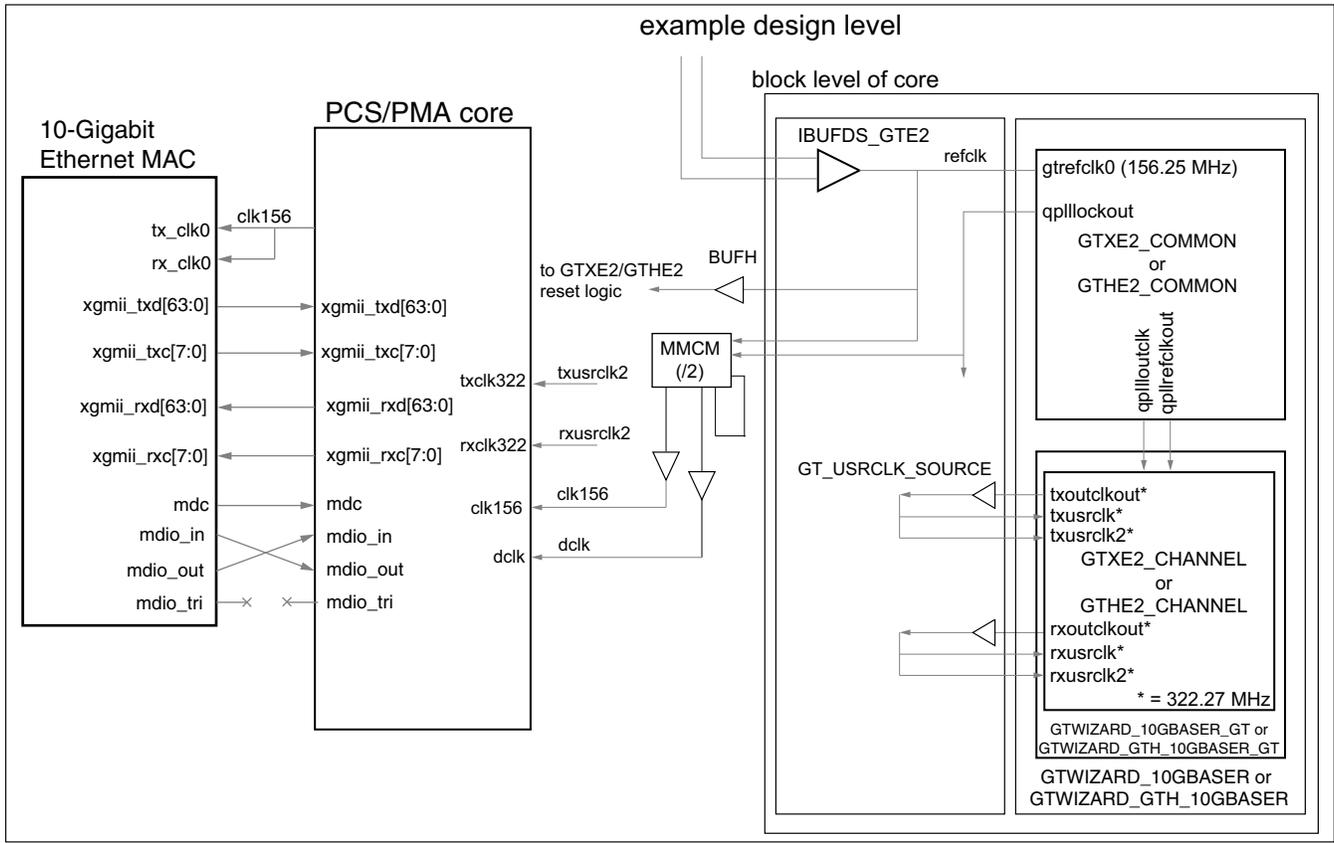
Figure 3-41: 10-Gigabit Ethernet MAC Core Integrated with PCS/PMA Core – Virtex-7 and Kintex-7 FPGAs
