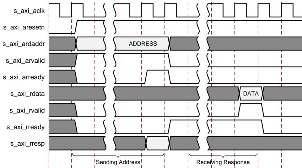
Figure 3-25: Management Register Read Timing
