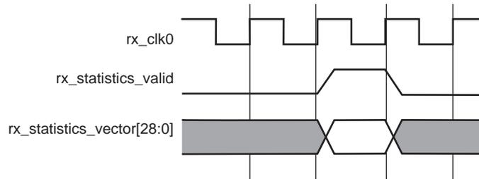
Figure 3-33: Receiver Statistics Output Timing
