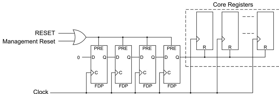
Figure 3-2: Reset Circuit for a Single Clock/Reset Domain
