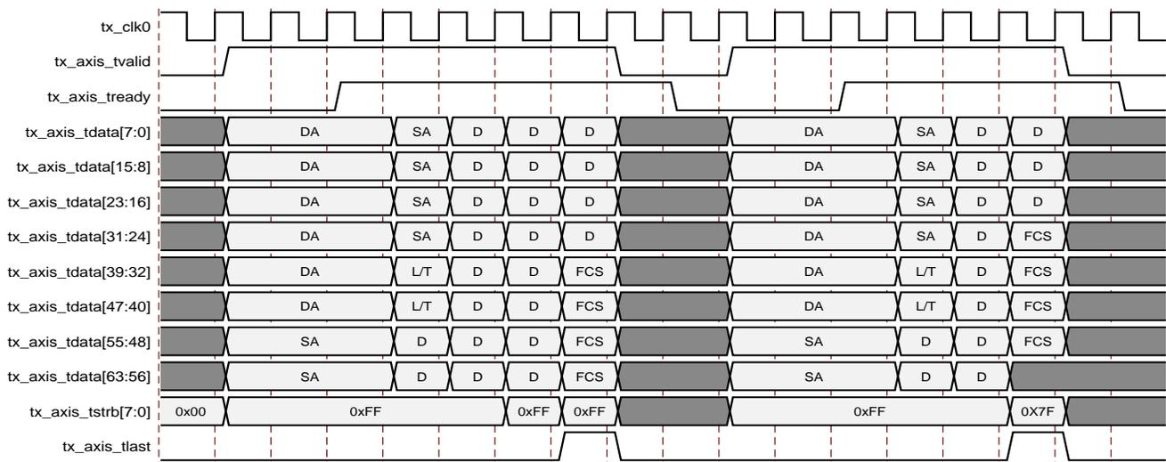
Figure 3-7: Transmission with In-Band FCS Passing
