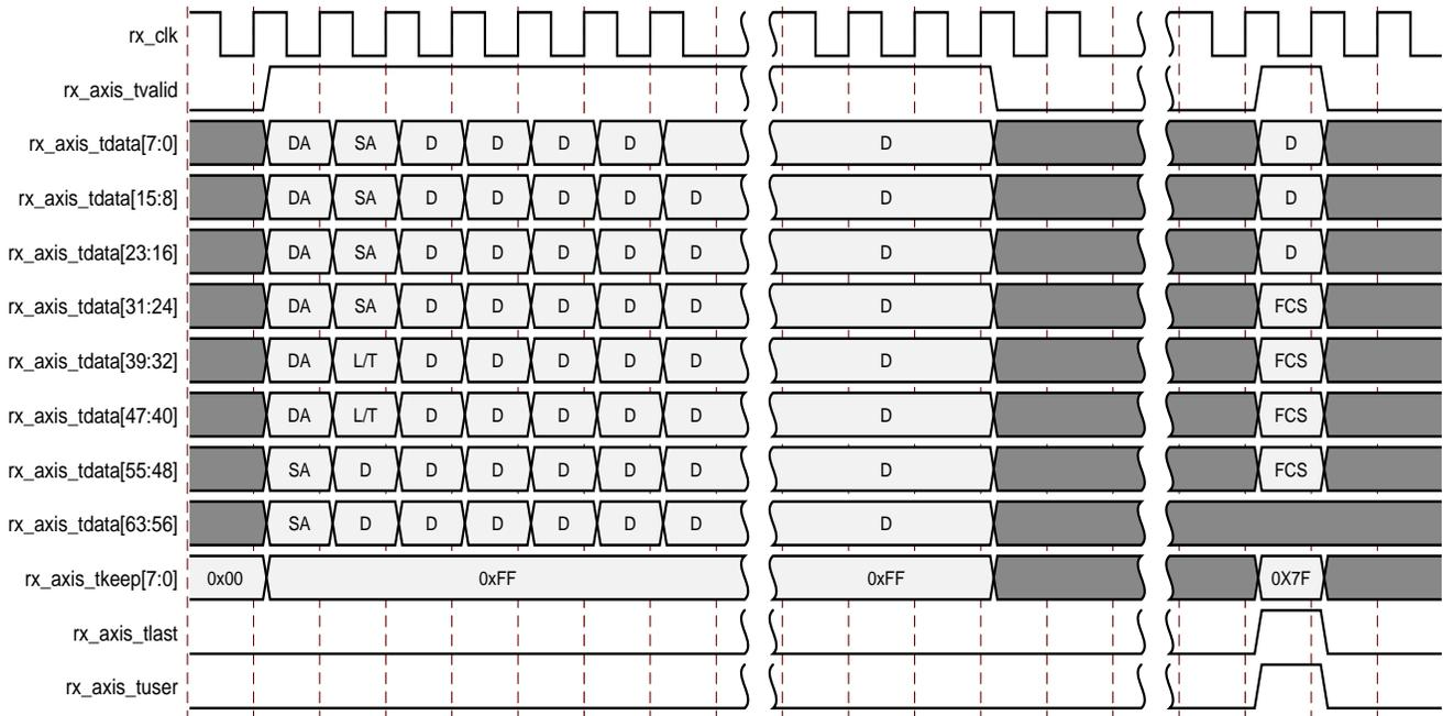
Figure 3-20: Frame Reception with In-Band FCS Passing
