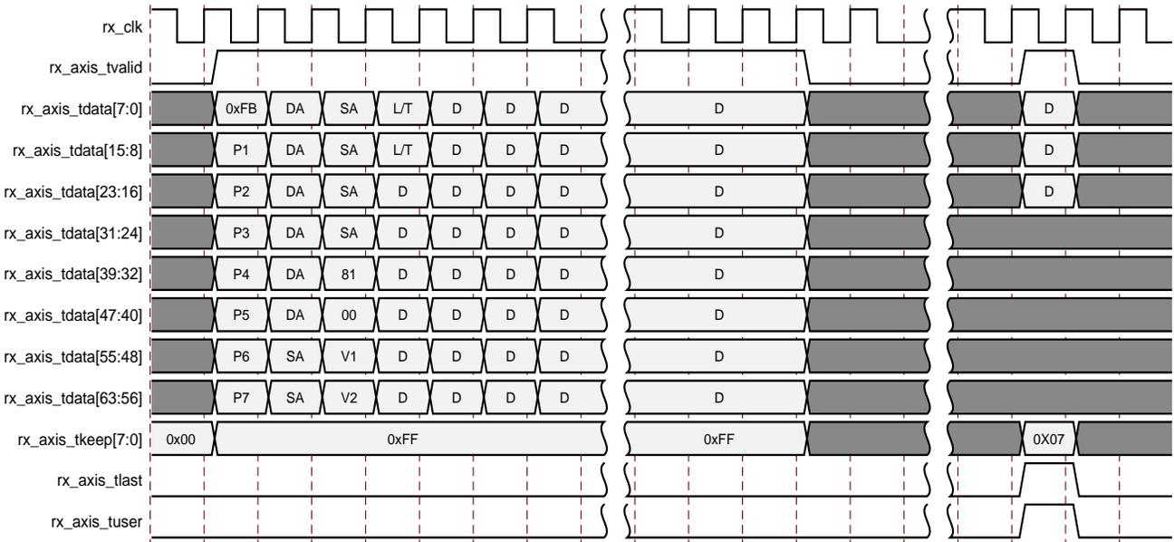
Figure 3-22: Frame Reception with VLAN Tagged Frames
