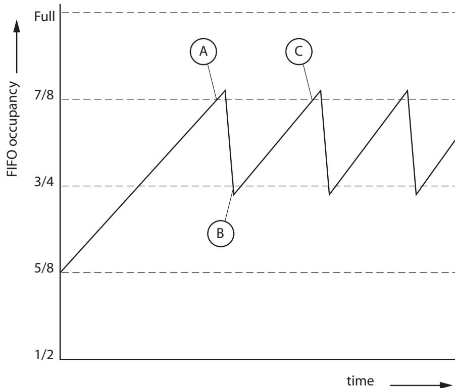
Figure 3-37: **Flow Control Implementation Triggered from FIFO Occupancy**
