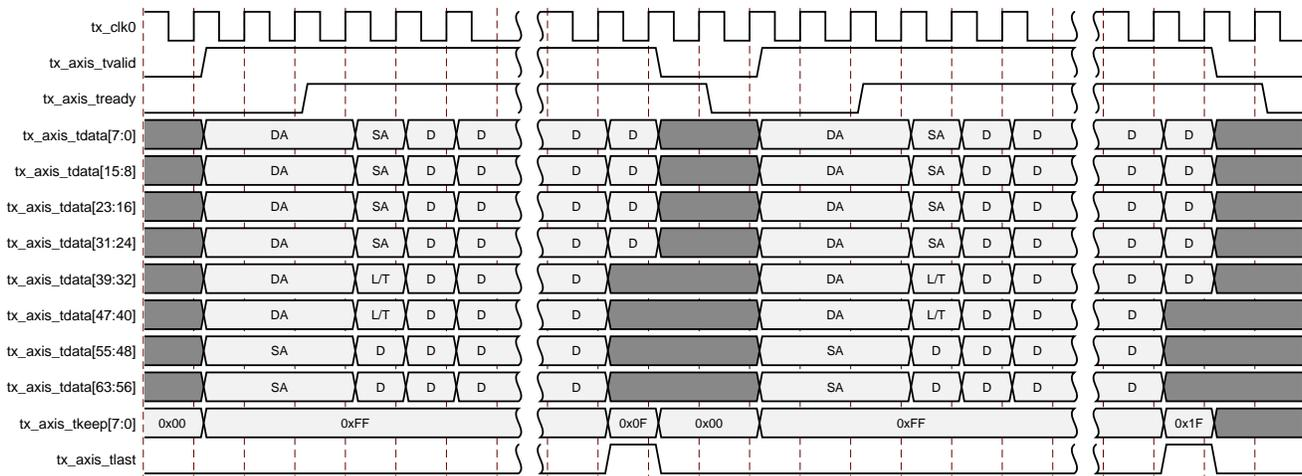
Figure 3-6: Frame Transmission
