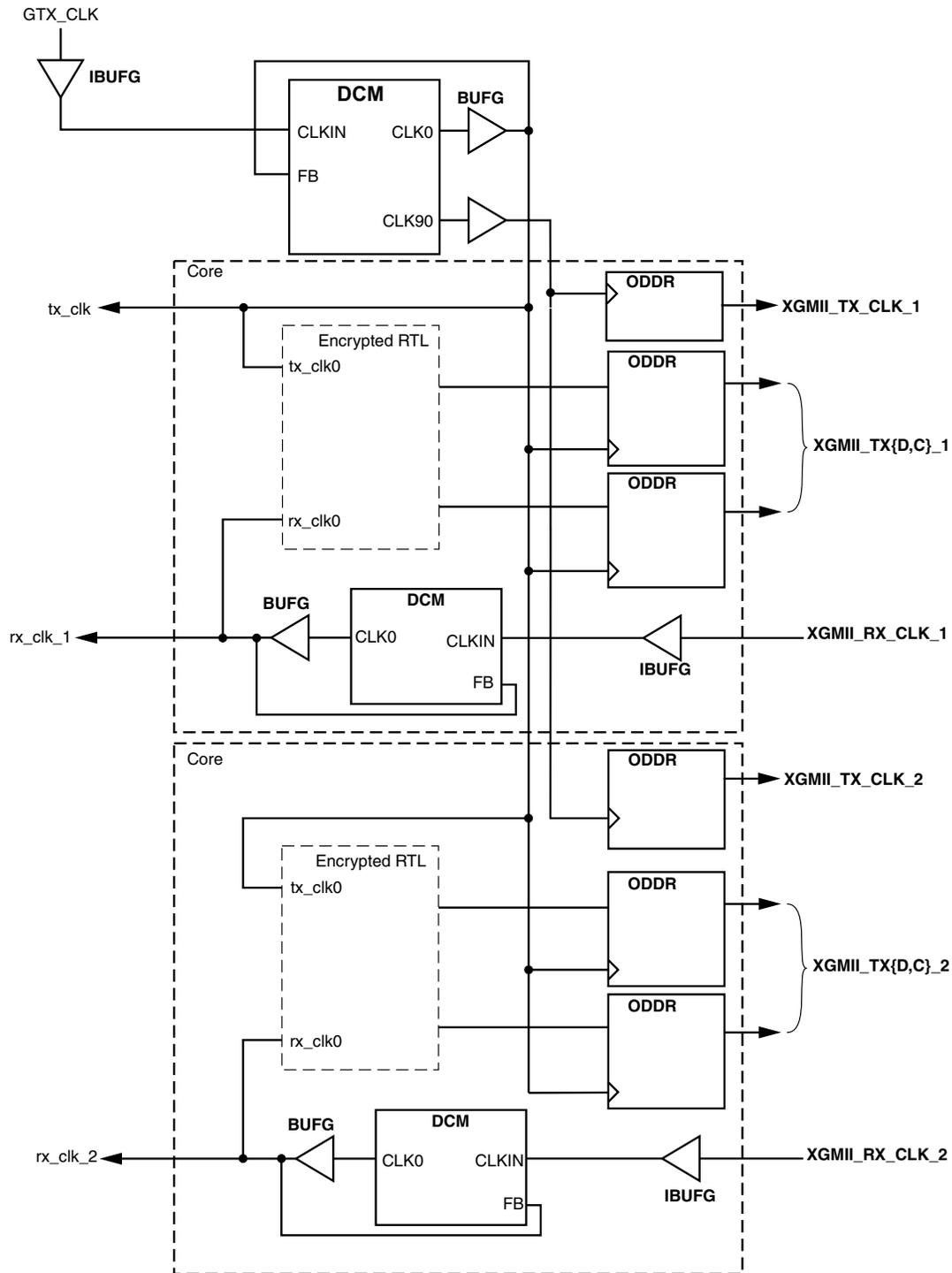
Figure 3-38: Clock Management, Multiple Instances of the Core with XGMII
