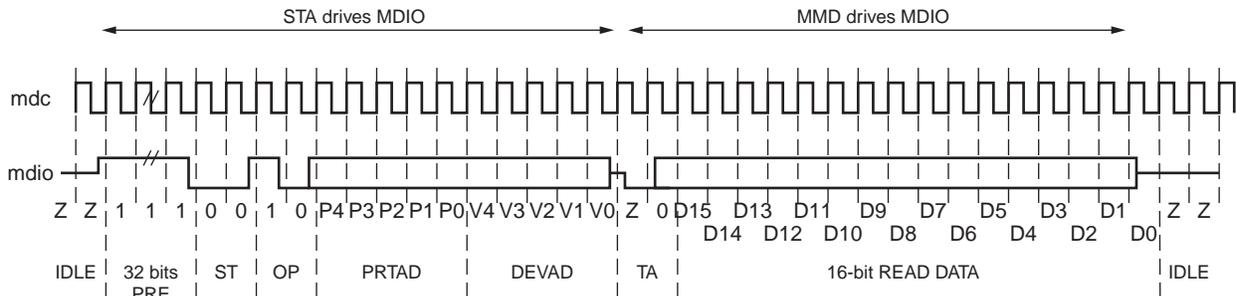
Figure 3-31: MDIO Read-and-Increment Transaction
