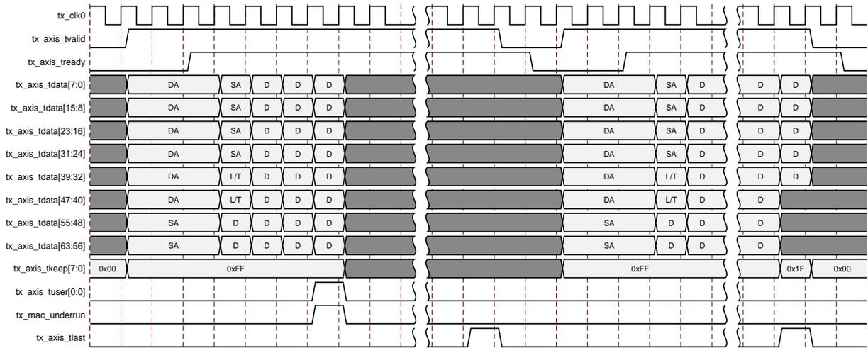
Figure 3-8: Frame Transfer Abort with `tx_axis_tuser` asserted
