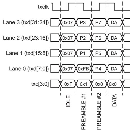
Figure 3-13: XGMII Frame Transmission of Custom Preamble
