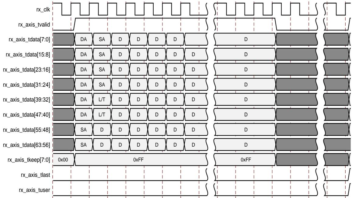
Figure 3-20: Frame Reception with In-Band FCS Passing
