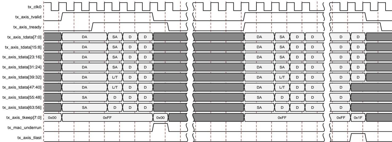
Figure 3-9: Frame Transfer Abort with tx\_axis\_tvalid deasserted
