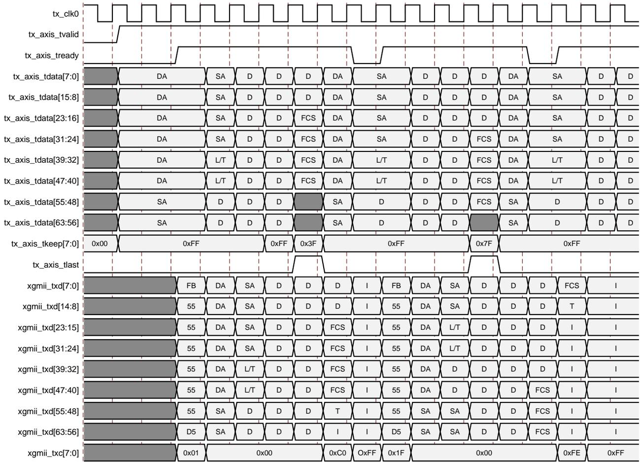
Figure 3-16: Back-to-Back Continuous Transfer on Transmit XGMII Interface
