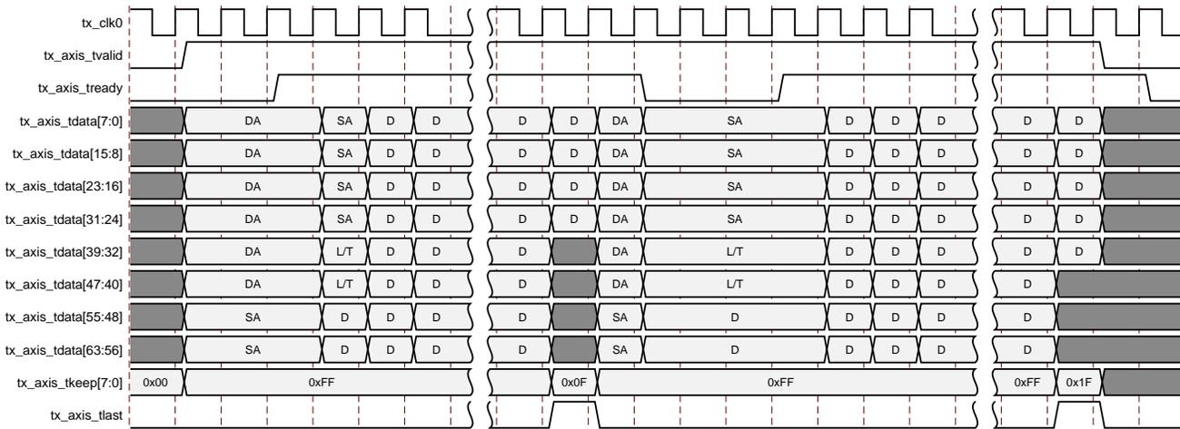
Figure 3-10: Back-to-Back Continuous Transfer on Transmit Client Interface
