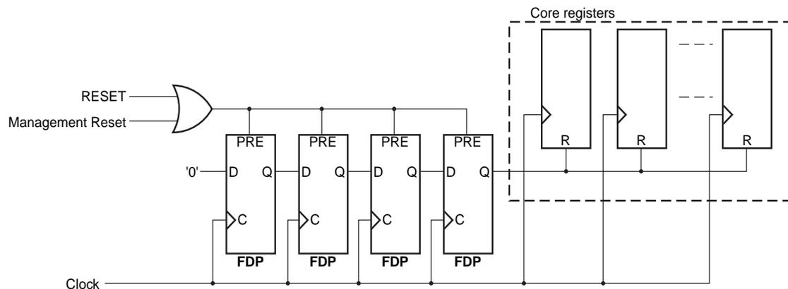
Figure 3-2: Reset Circuit for a Single Clock/Reset Domain
