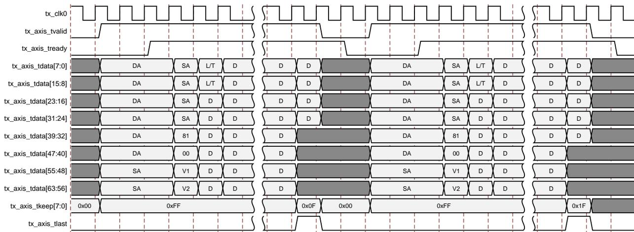
Figure 3-14: VLAN Tagged Frame Transmission
