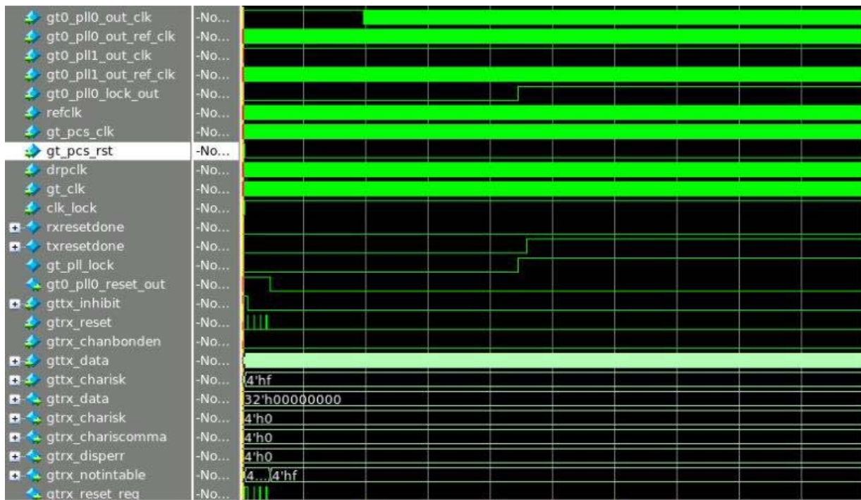
Figure C-6: GT Interface Signals
