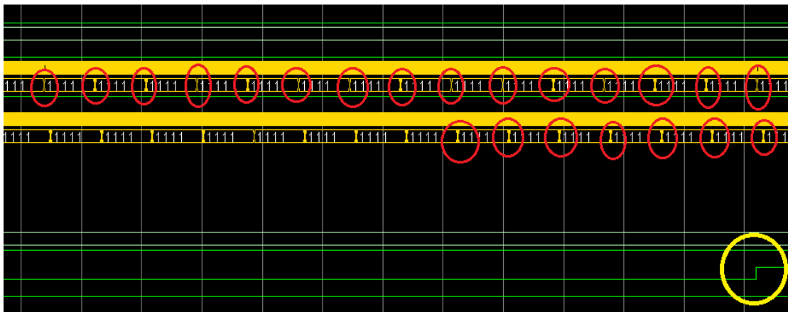
Figure C-4: port_initialized and link_initialized Signals (Figure C-3 Enlarged)
