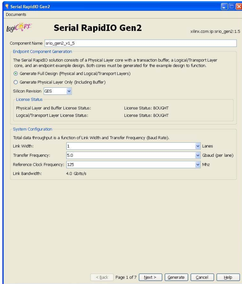
Figure 7-1: Serial RapidIO Gen2 Main Configuration Screen
