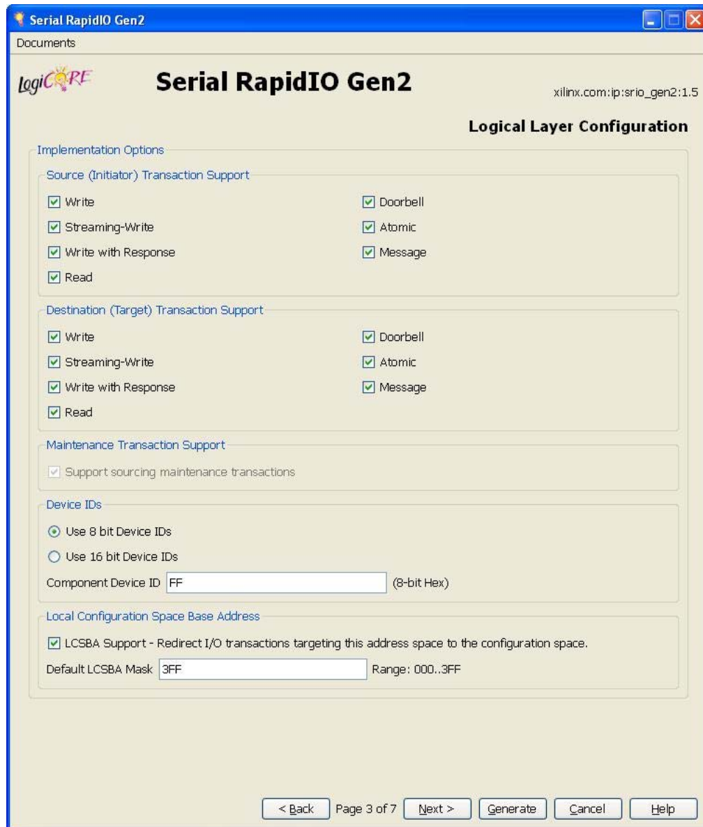
Figure 7-3: Logical Layer Configuration Screen
