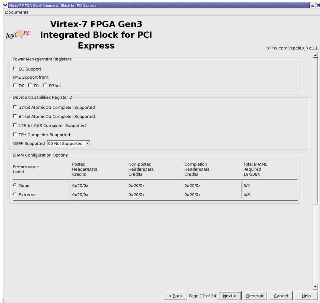
Figure 7-12: Page 12: Power Management Registers
