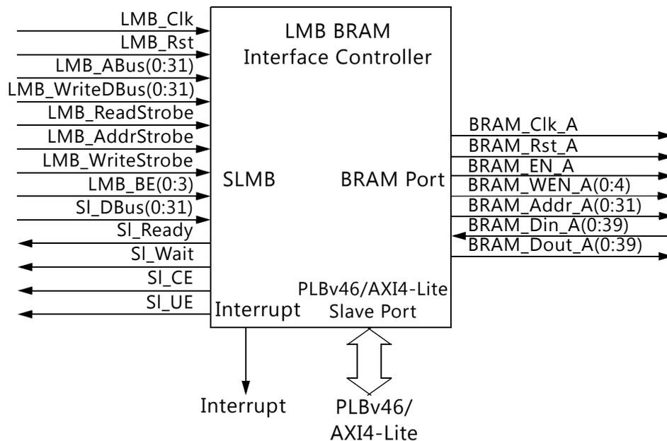
Figure 1-1: LMB BRAM Interface Controller Block Diagram
