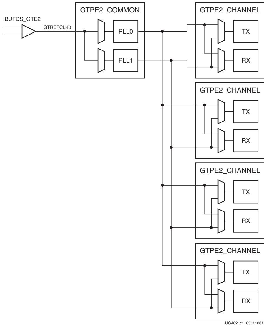
Figure 2: **Serial Transceiver REFCLK Sourcing**
