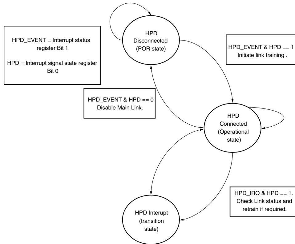
Figure 4-8: HPD Event Handling in Source Core
