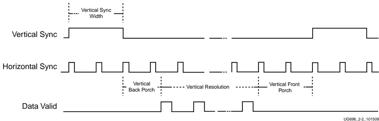
Figure 4-17: User Interface Vertical Timing
