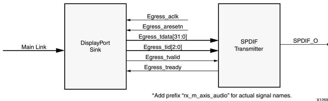
Figure 4-16: Audio Data Interface of DisplayPort Sink System
