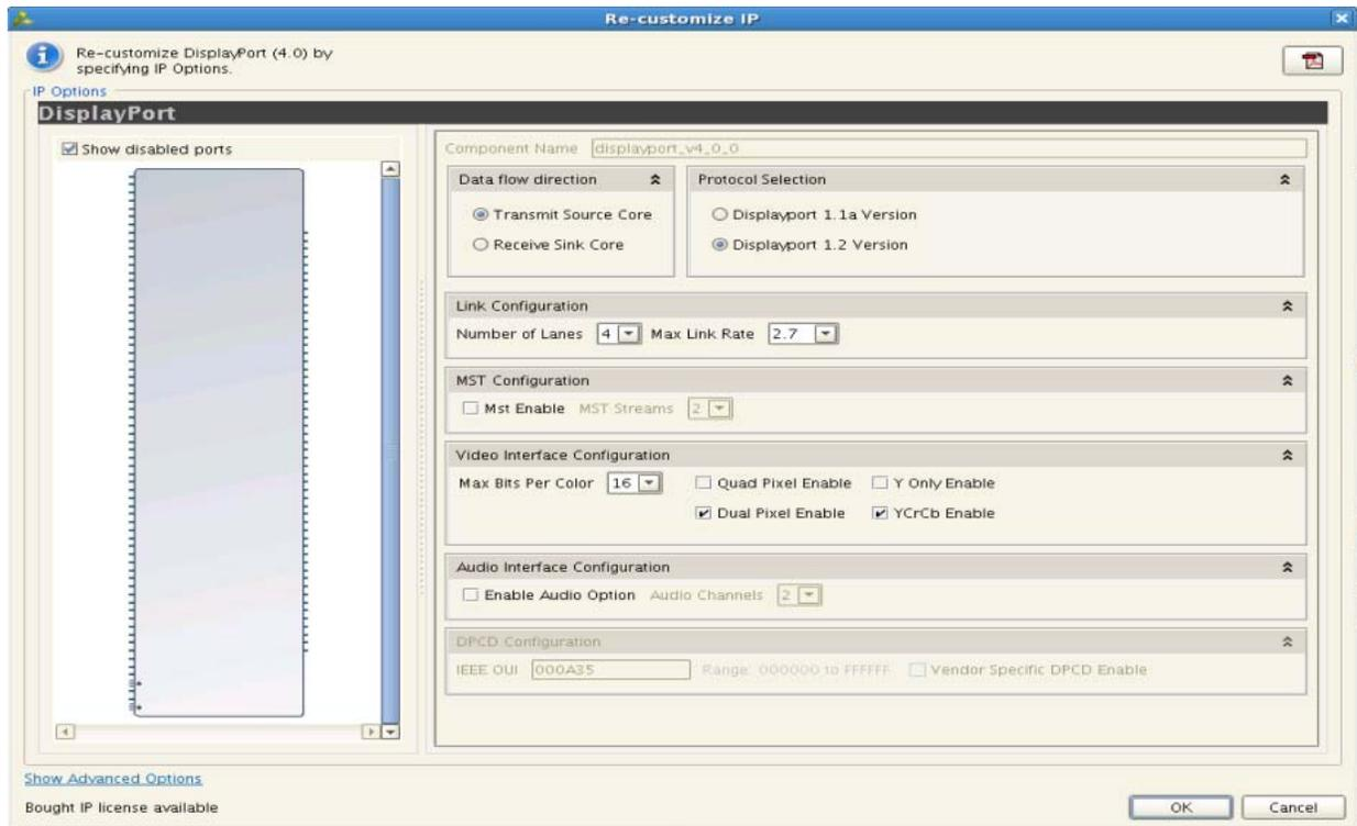
Figure 5-1: DisplayPort IP Customization Main Screen
