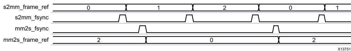
Figure 2-23: Example Genlock Timing
