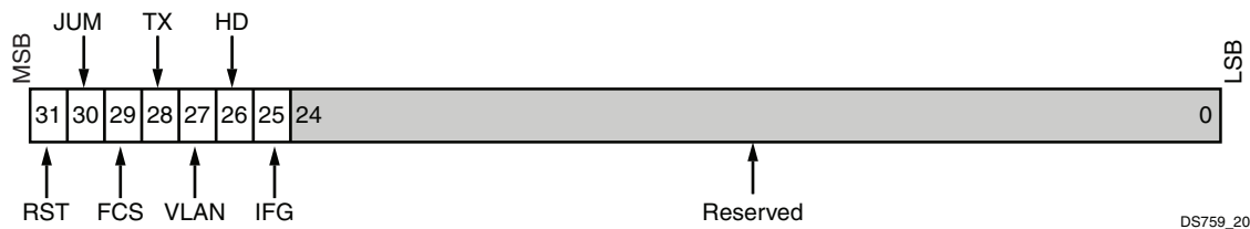
Figure 2-49: TEMAC Transmit Configuration Register (offset 0x408)
