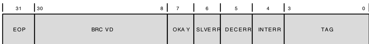
Figure 3-6: Special S2MM Status Word Layout (IBTT Mode Enabled)
