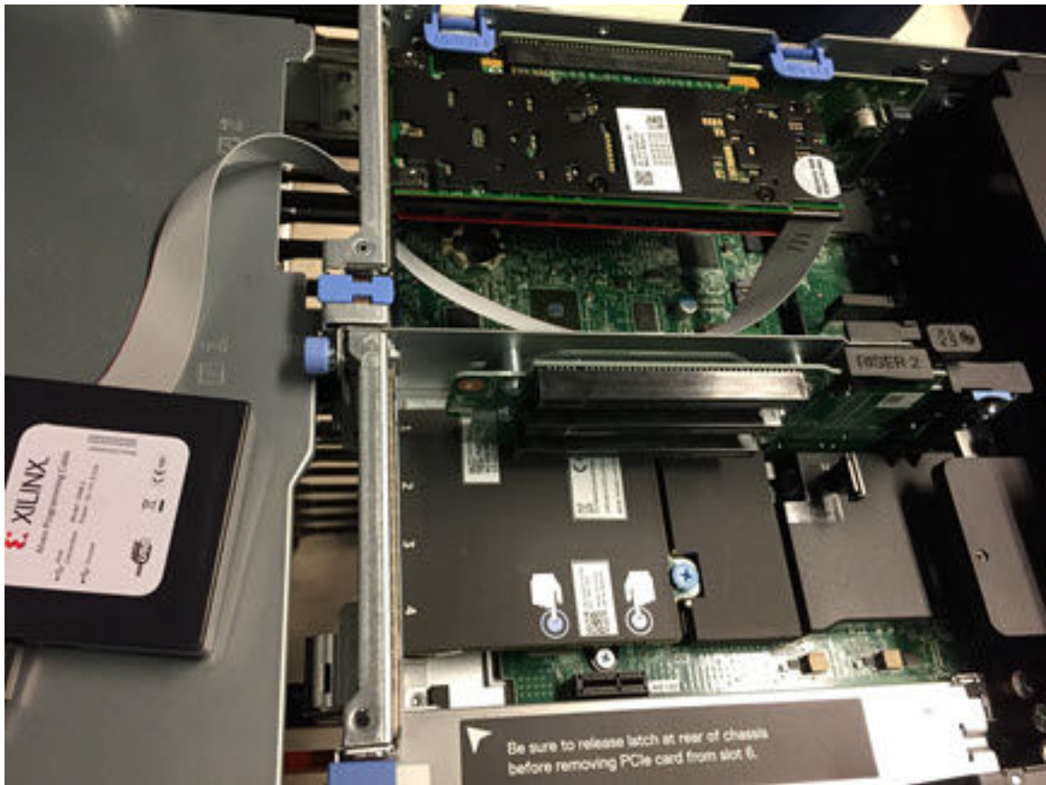
Figure 8: Installed Alveo Data Center Accelerator Card Connected to Alveo Programming Module – Side View
