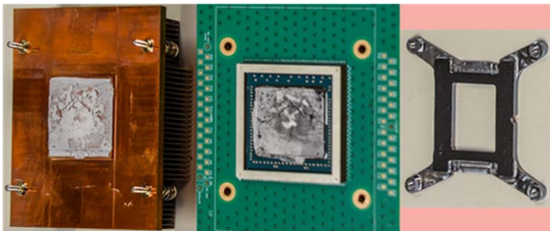
Figure 1-13: Example of Heat Sink for VU13P-FIGD2104 with PCM780SP
