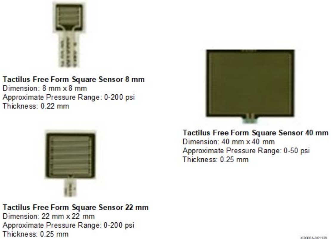
Figure A-4: Pressure Sensor – Tactilus Free Form Square Sensors
