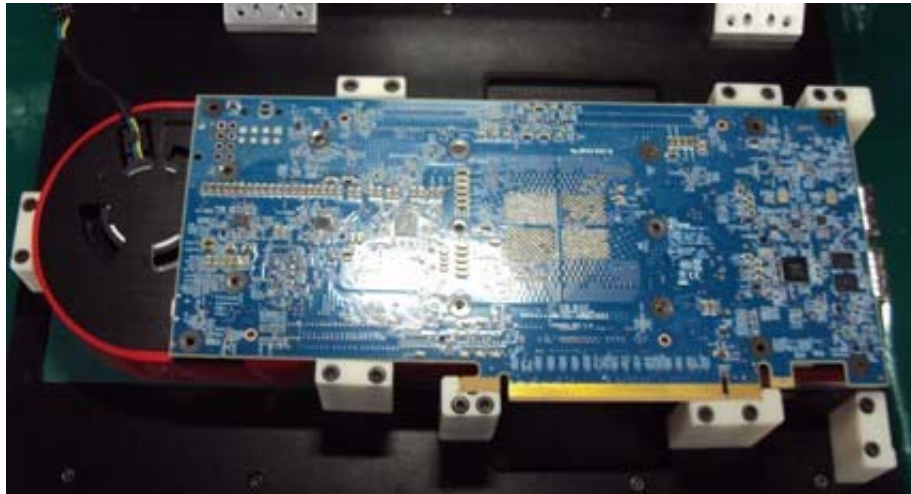
Figure A-17: Heat Sink with PCBA on top
