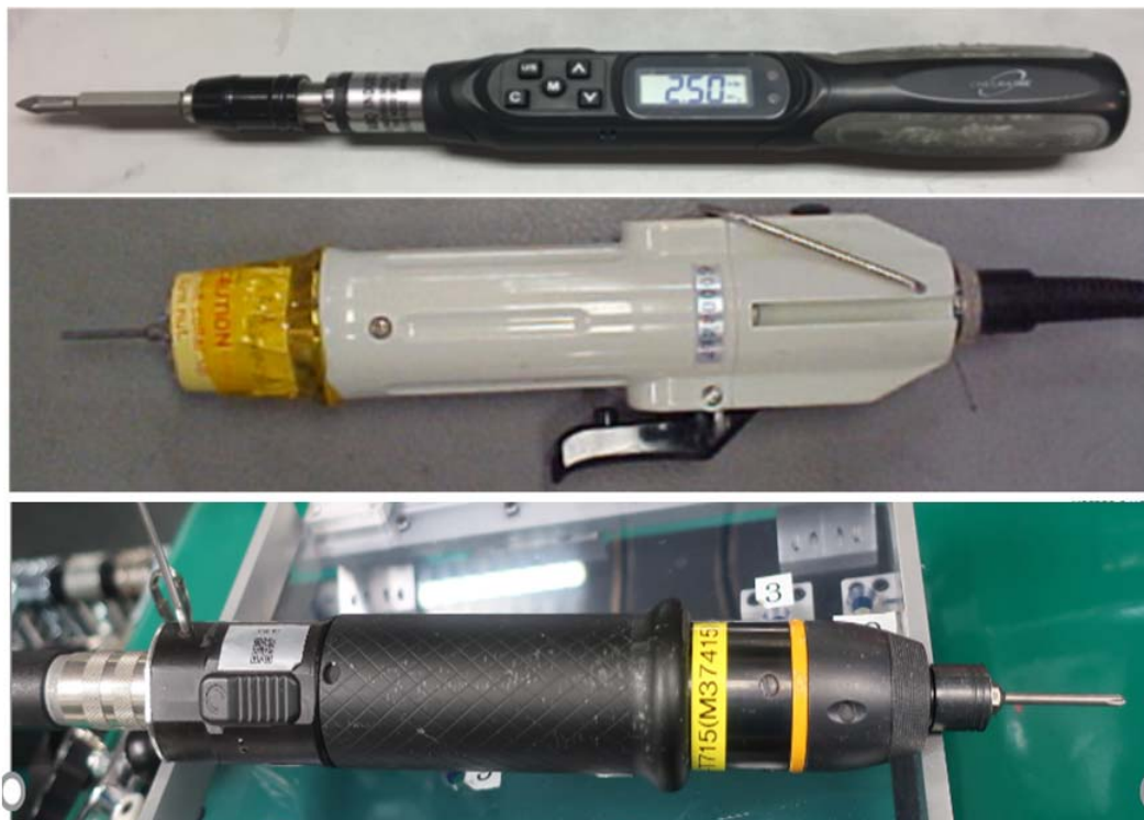
Figure A-1: Digital Torque Screwdriver (Top), Hios CL 2000 (Middle), and Hios CL 2000 (Bottom)
