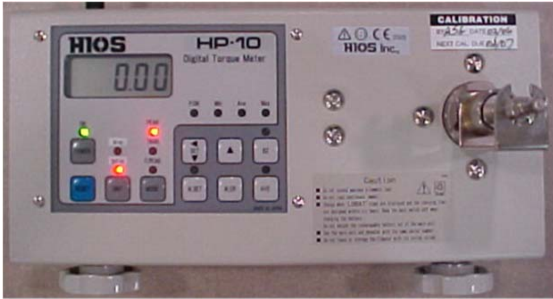
Figure A-2: Screw Torque Calibrator – Hios HP-10
