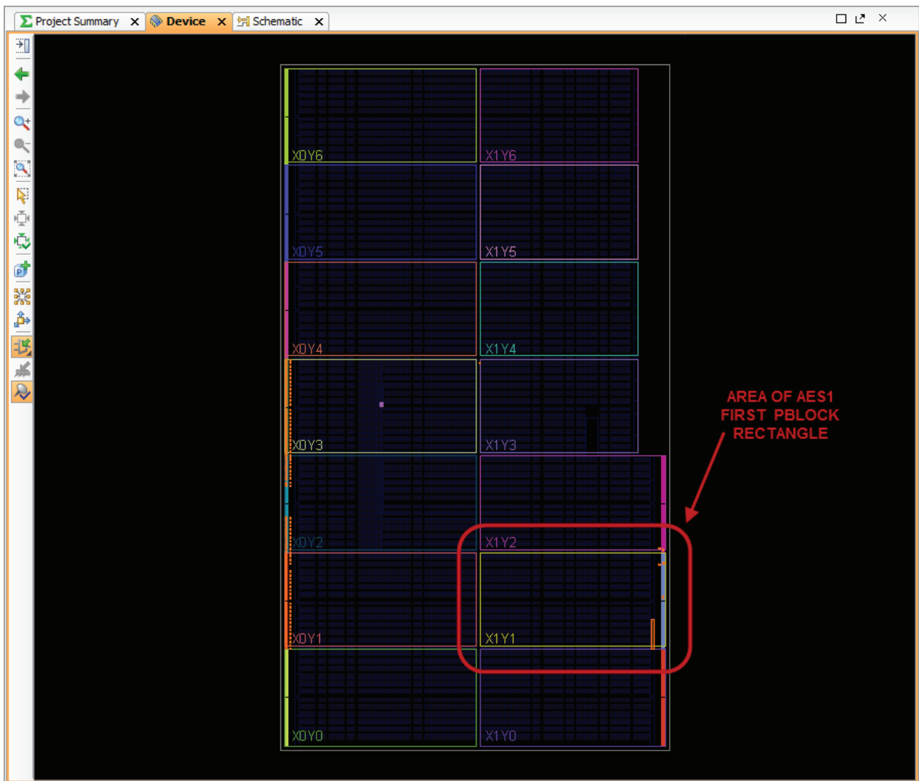
Figure 3-15: XC7K325T-2FFG900 Whole View Reference for First Pblock
