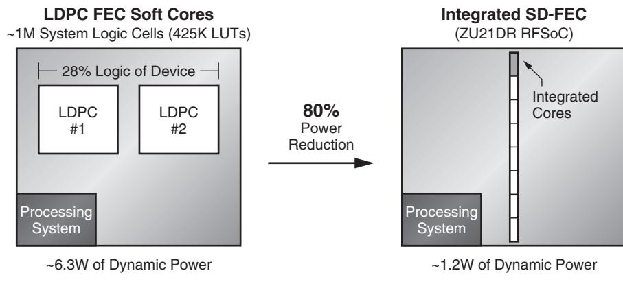
Figure 5: Power Comparison of Integrated SD-FEC versus Soft LDPC Decoder
