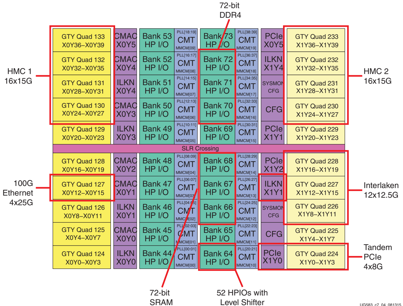
Figure 7-4: VU7P Floorplan for Migration from VU125
