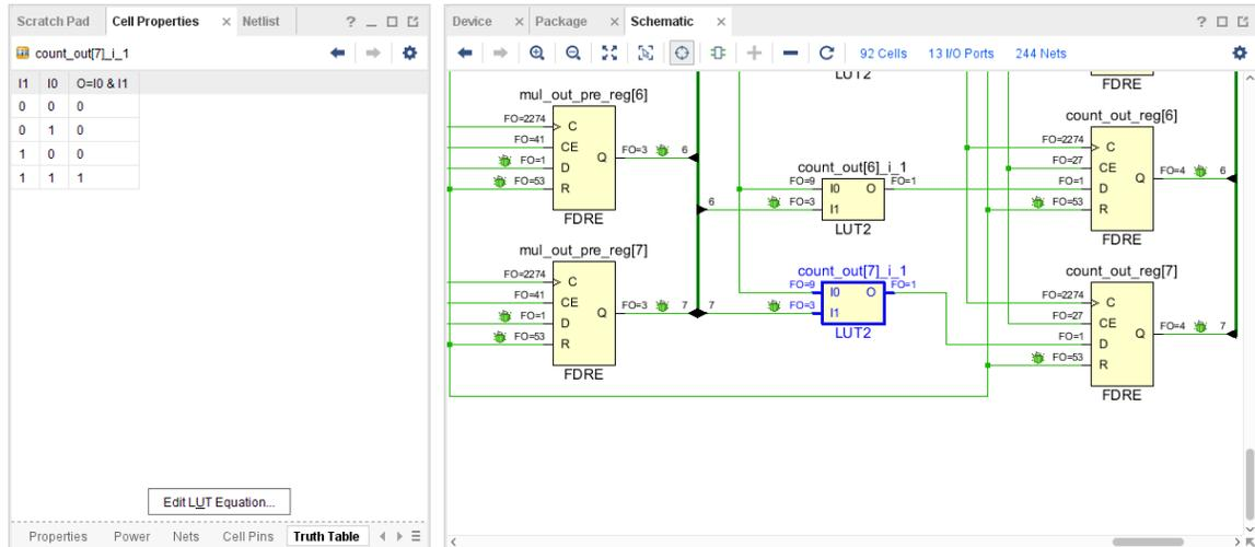
This command selects the LUT2 that drives the `count_out_reg[7]` register, which drives LED 7 on the KCU105 board. The only inputs are `tog_state_reg` for pin I0 and `mul_out_pre_reg[7]` for pin I1. You need to replace the LUT2 with a 3-input LUT and connect the output of counter register `divClk_reg[24]` to the additional input pin.
