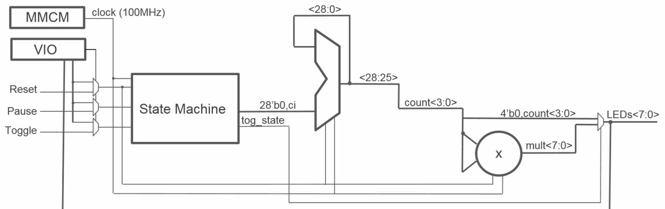
In this design, a mixed-mode clock manager (MMCM) is used to synthesize a 100 MHz clock from the 300 MHz clock provided by the board.
