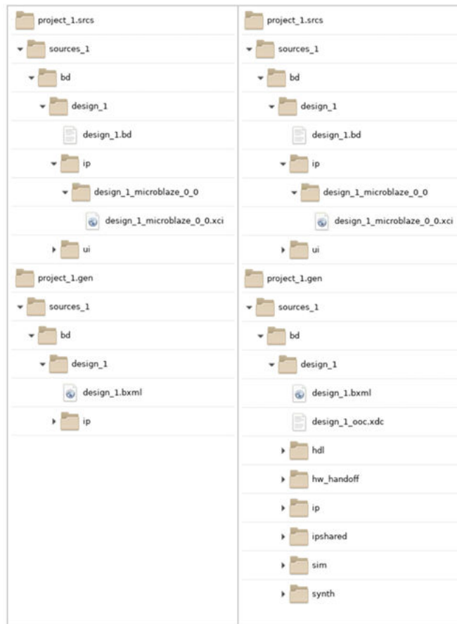
Figure 134: Directory Structure for Project IP and BD Files Before (Left) and After (Right) Generate Design
