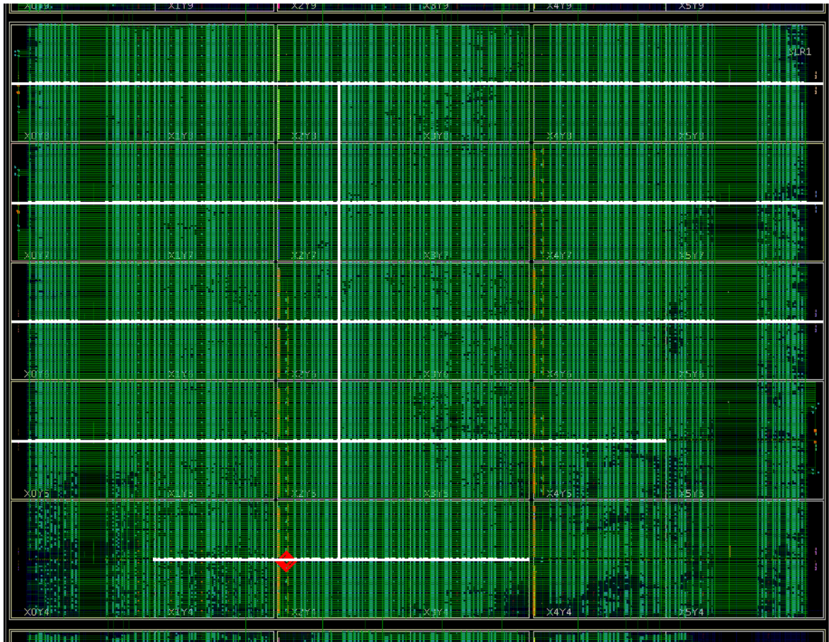
Figure 51: High Fanout Clock Spanning an SLR
