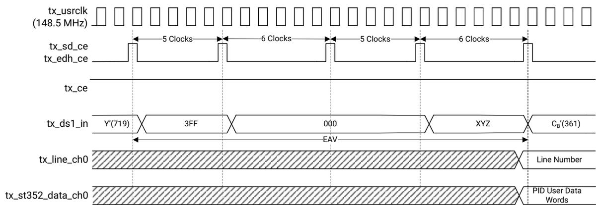
Figure 3-2: SD-SDI TX Timing Diagram
