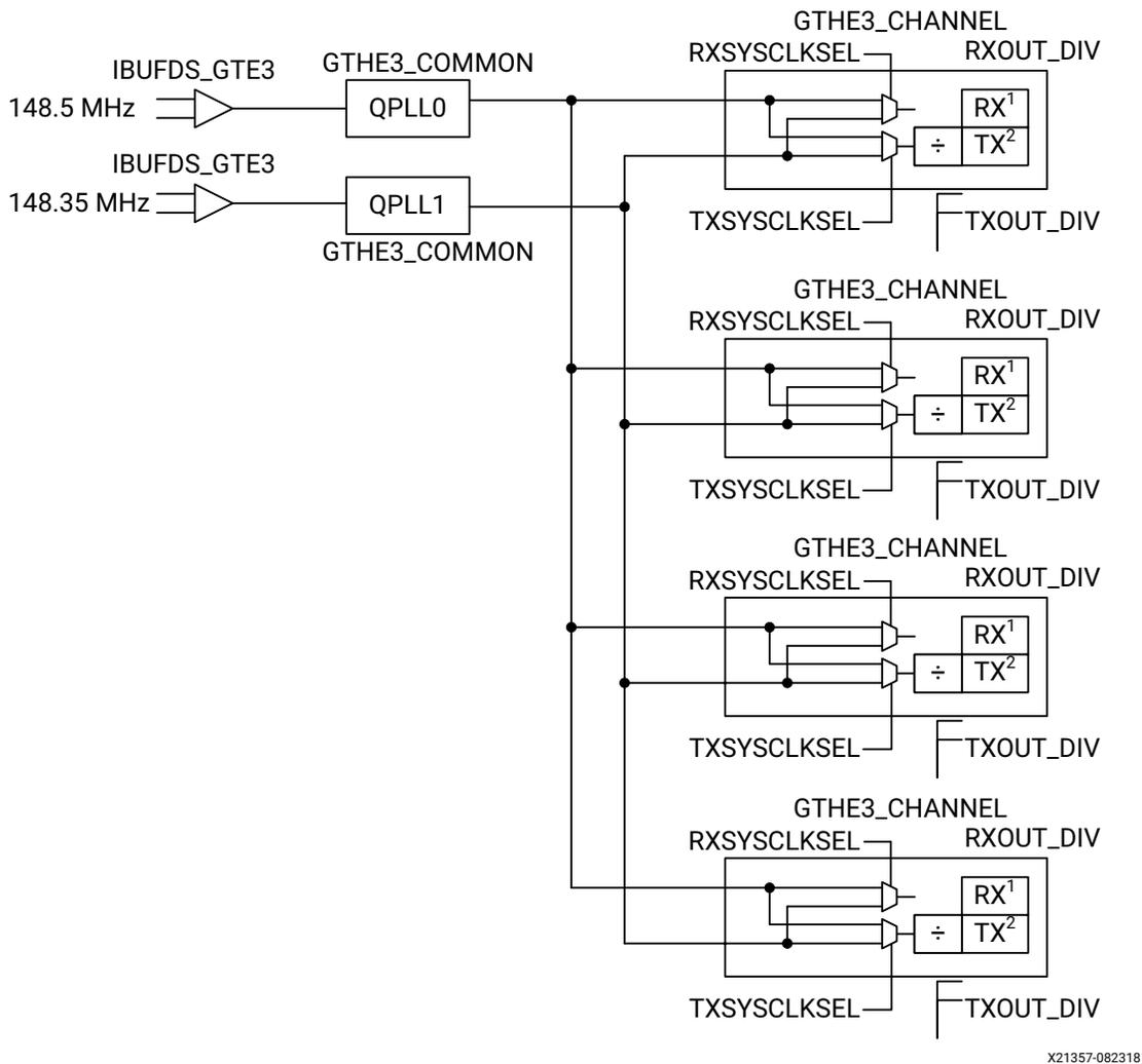
Figure 2-4: UltraScale/UltraScale+ GTH PLL Configuration for SMPTE UHD-SDI Core
