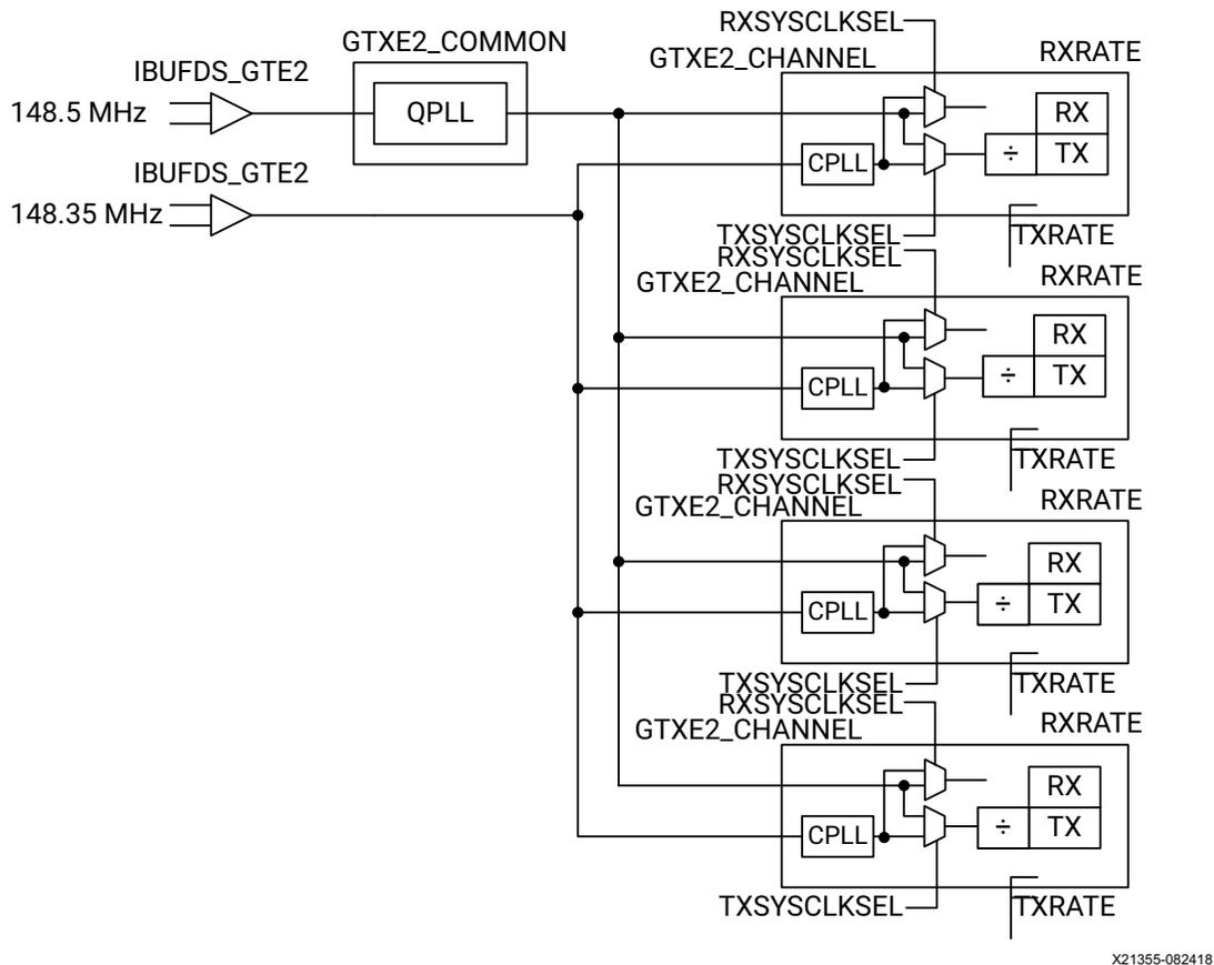
Figure 2-2: GTX PLL Configuration #2
