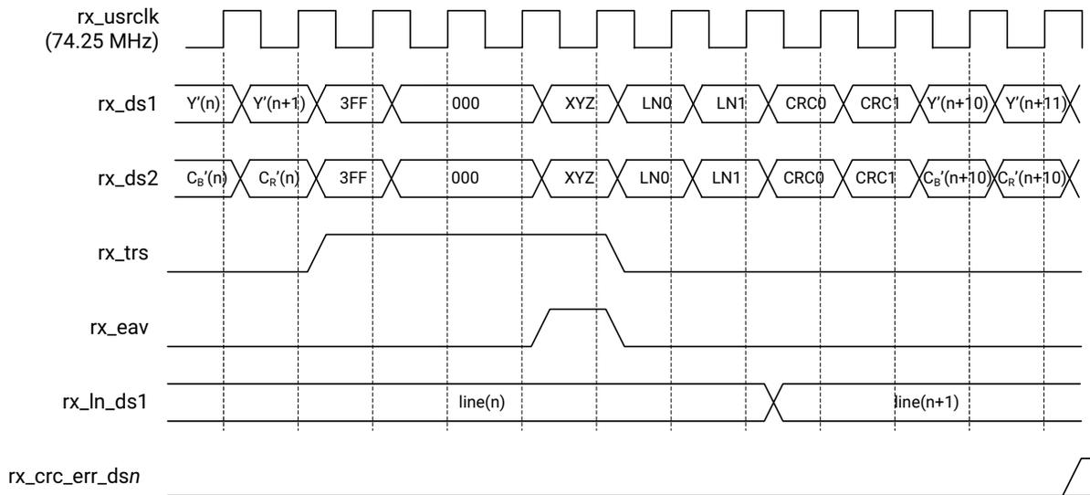
Figure 3-3: HD-SDI RX Timing Diagram
