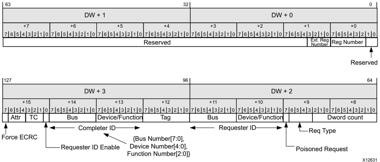
Figure 3-43: Requester Request Descriptor Format for Configuration Requests
