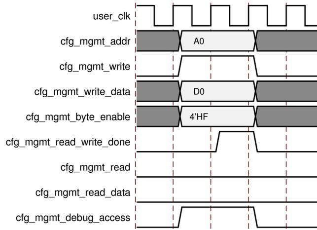
Figure 3-78: `cfg_mgmt_debug_access`
