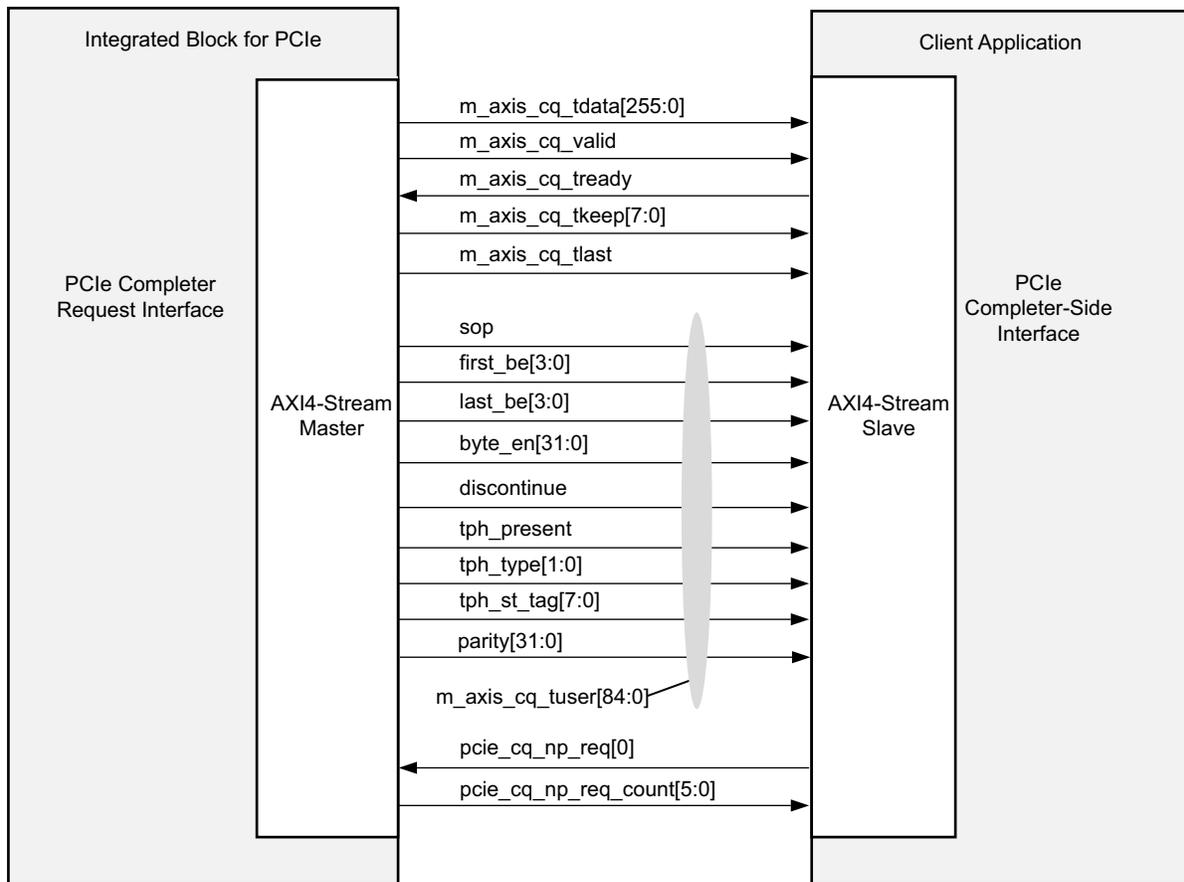
Figure 3-18: Completer Request Interface Signals
