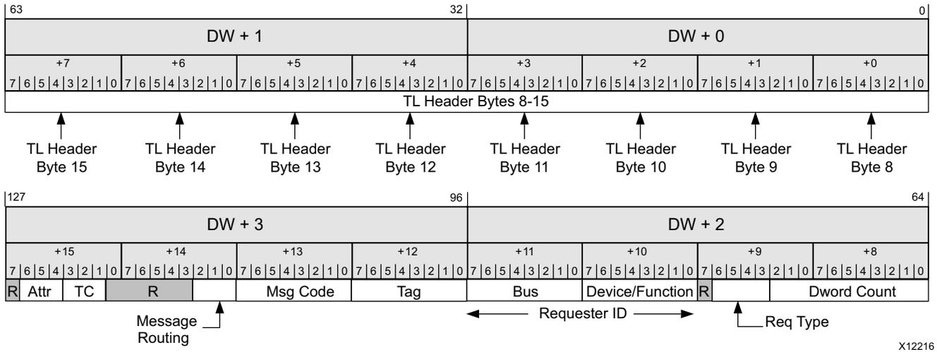
Figure 3-21: Completer Request Descriptor Format for ATS Messages
