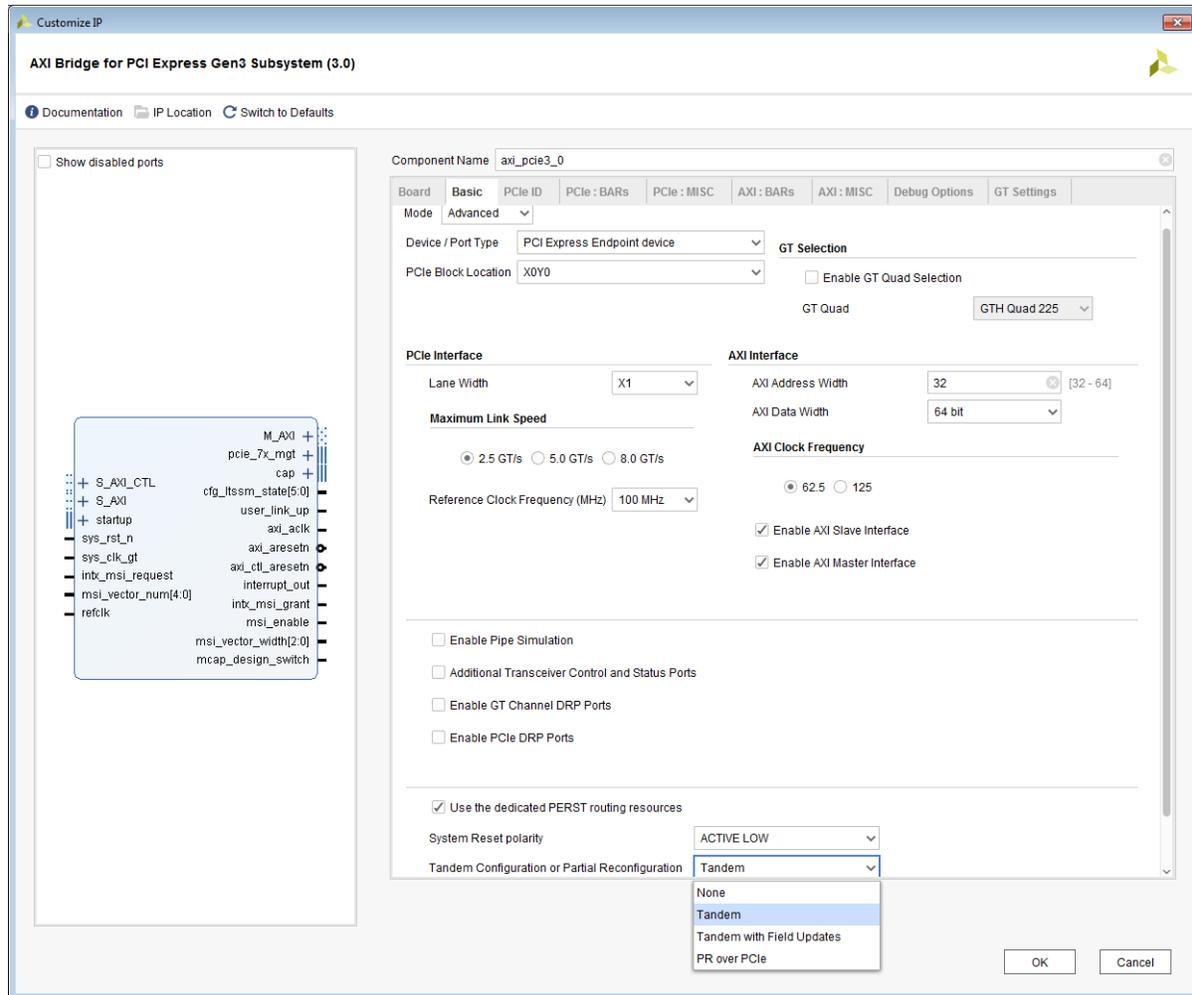
Figure 3-10: Tandem PCIe
