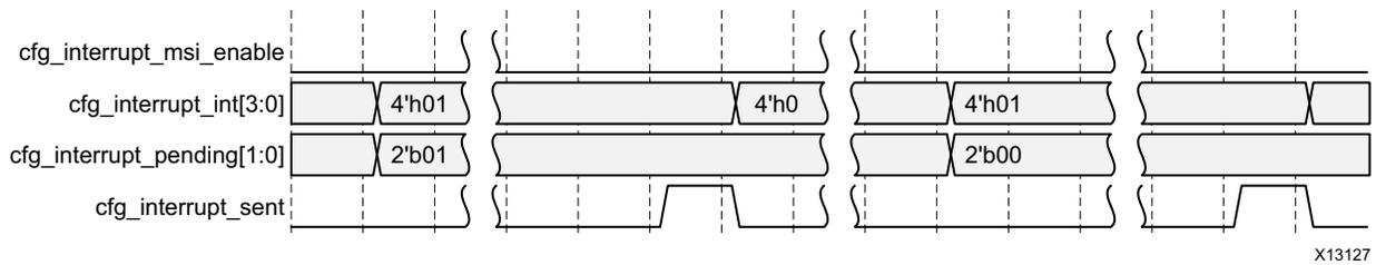
Figure 3-72: Legacy Interrupt Signaling
