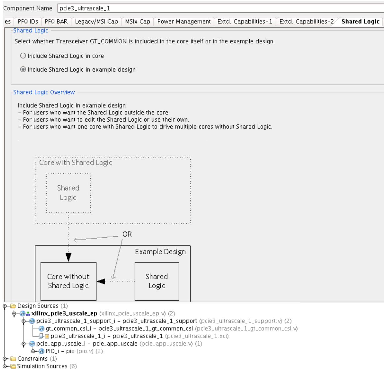
Figure 3-2: Shared Logic in the Example Design
