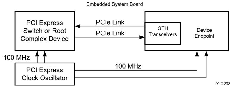
Figure 3-15: Embedded System Using 100 MHz Reference Clock
