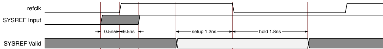
Figure 3-8: SYSREF Timing using Negative Edge Sampling
