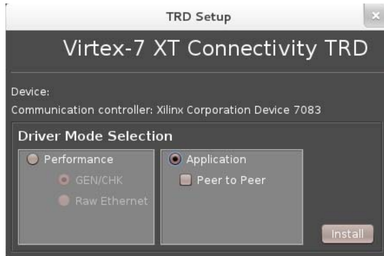
Figure 2-19: Application Mode Driver Installation
