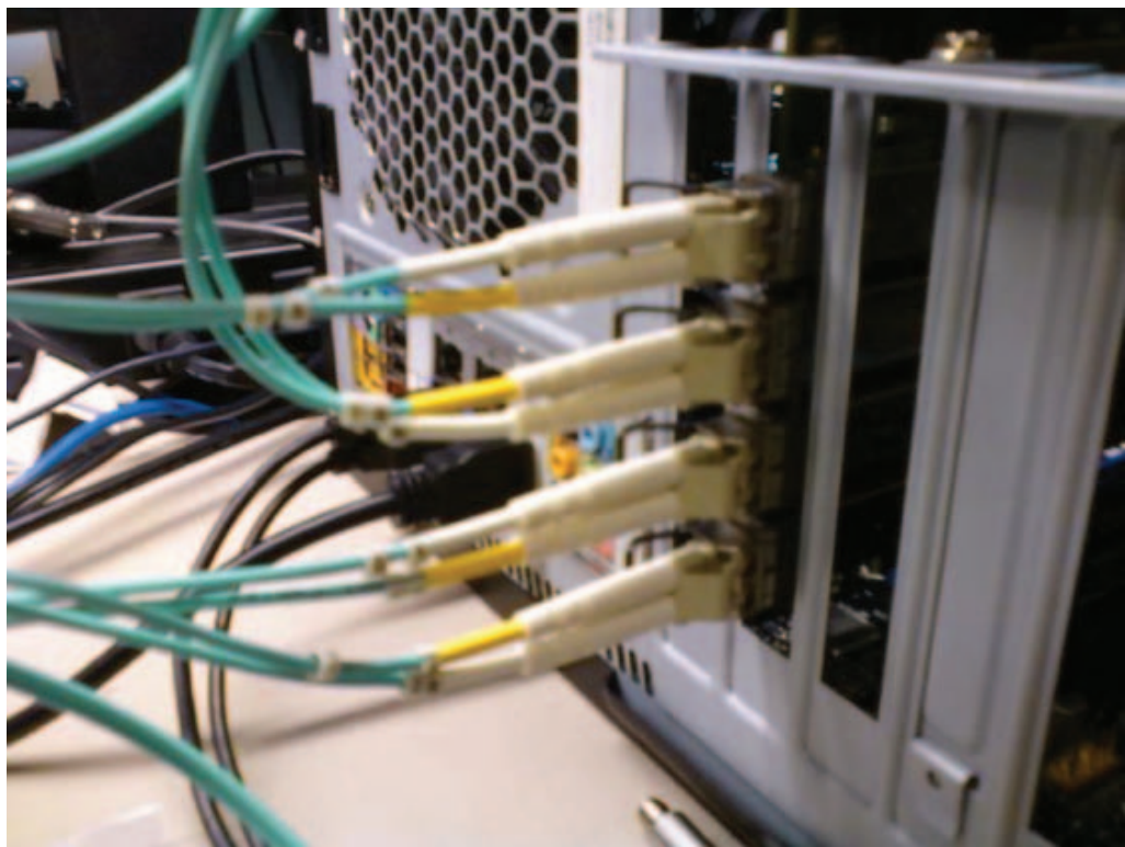
Figure 2-3: Setup with Fiber Optic Cable Installed in PC Chassis
