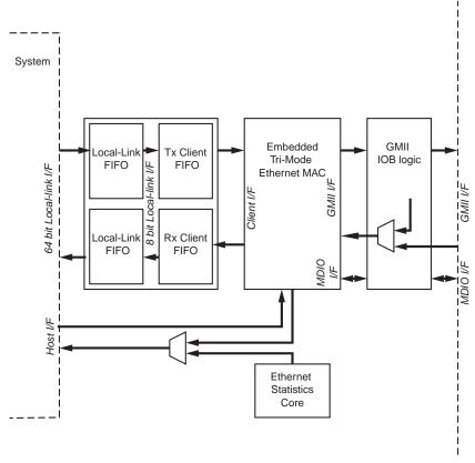
Figure 4: Embedded Tri-Mode Ethernet MAC FPGA Block Diagram
