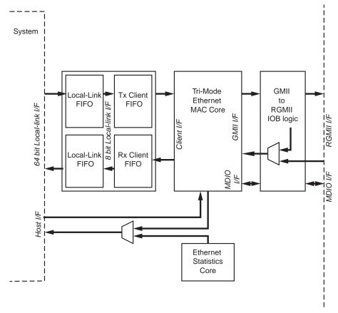
Figure 3: Tri-Mode Ethernet MAC FPGA Block Diagram
