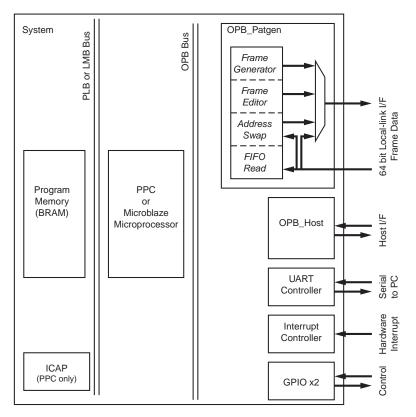
Figure 5: Microprocessor System Block Diagram
