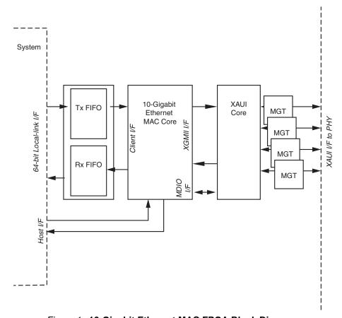
Figure 1: 10-Gigabit Ethernet MAC FPGA Block Diagram
