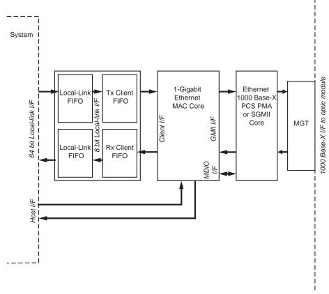
Figure 2: 1-Gigabit Ethernet MAC FPGA Block Diagram
