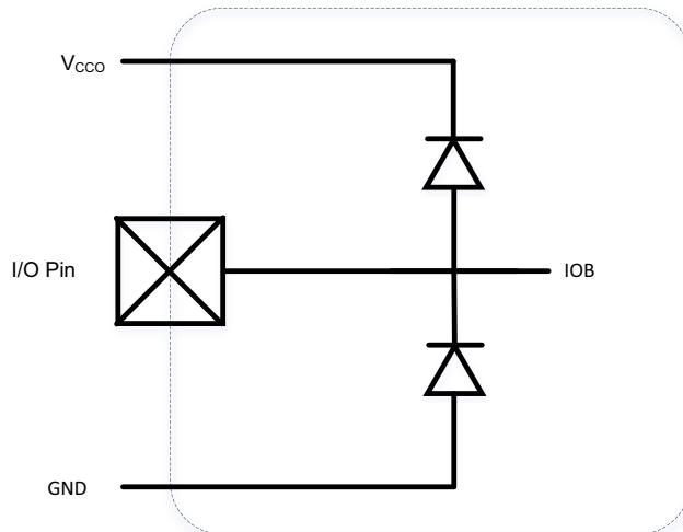
Figure 1: Xilinx FPGA I/O with Clamp Diodes
