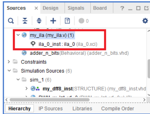
Figure 214: ILA IP Configured and Added to Project
