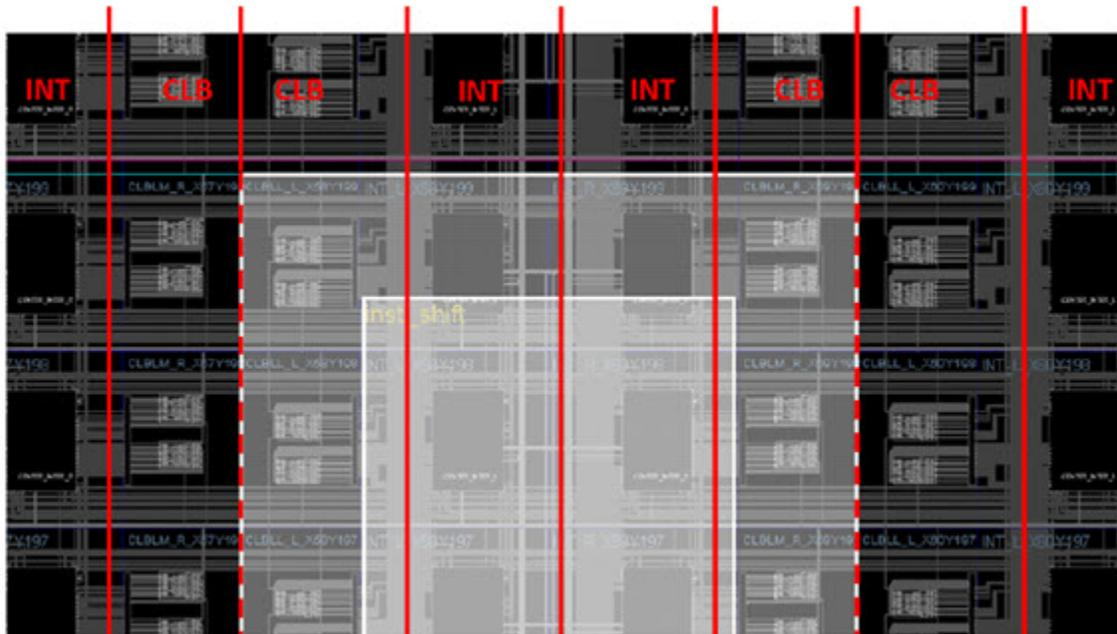
The RP Pblock must include all reconfigurable element types within the shape drawn. In other words, if the rectangle selected encompasses CLB (Slice), block RAM, and DSP elements, all three types must be included in the Pblock constraints. If one of these is omitted, a DRC is triggered with an alert that a split interconnect situation has been detected.
