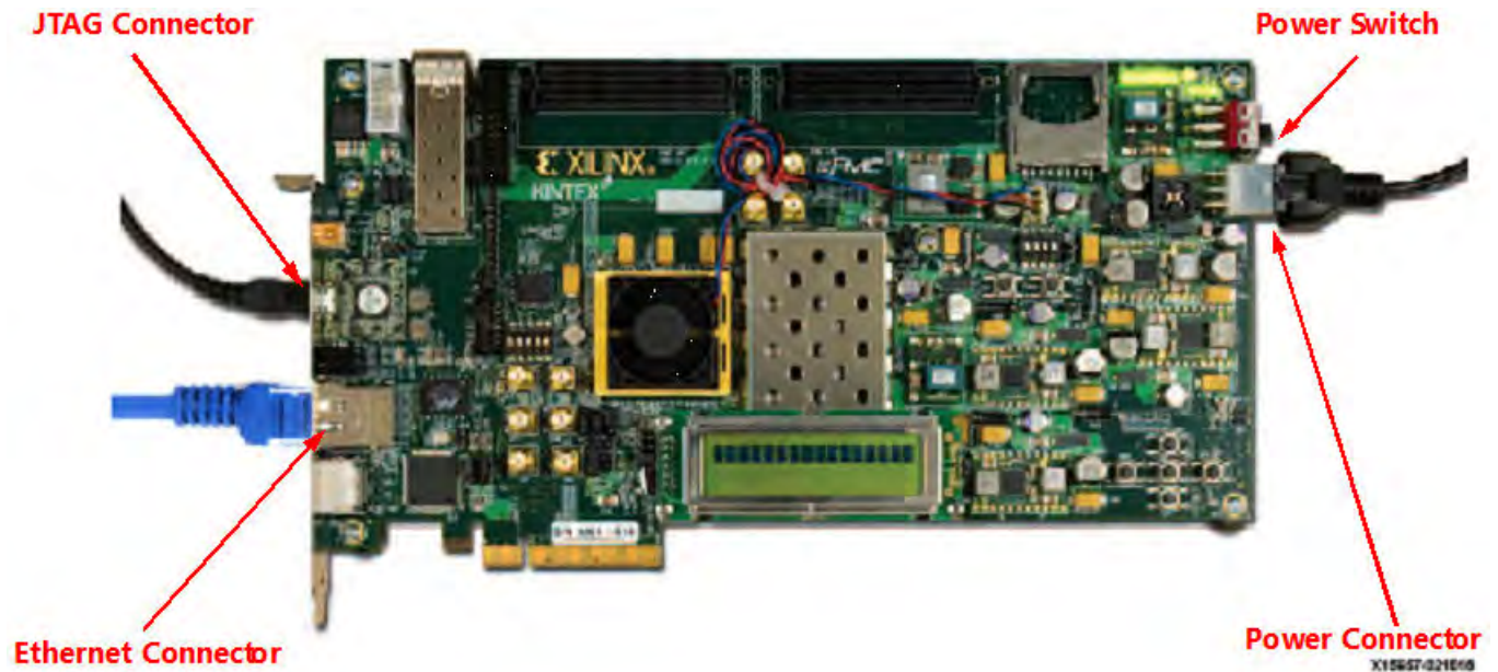
Figure 122: KC705 Board Ethernet Connections
