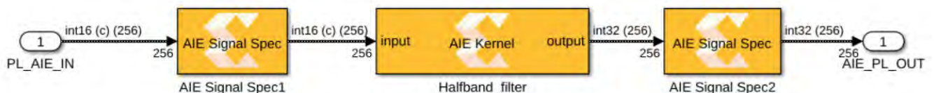
Figure 283: AIE Signal Spec Block Connected to AI Engine Subsystem
