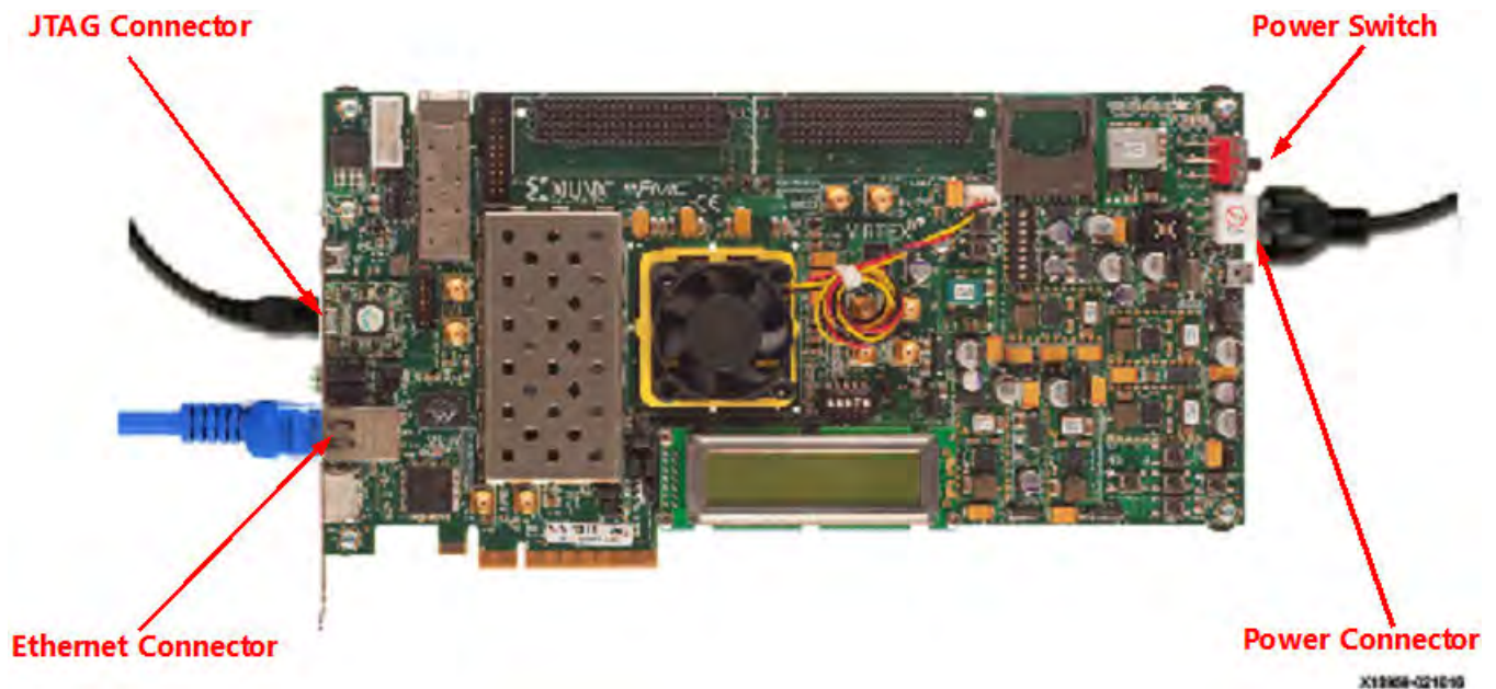
Figure 123: VC705 Board Ethernet Connections
