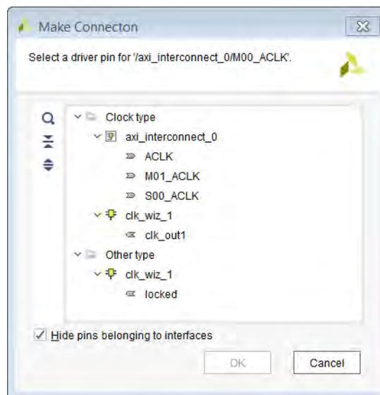
Selecting the appropriate clock source makes the connection between the clock source and the port or pin.
