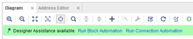
2. Click **Run Block Automation** to configure a basic processor sub-system. The processor sub-system is created which includes commonly used IP in a sub-system such as block memory controllers, block memory generator and a debug module.
