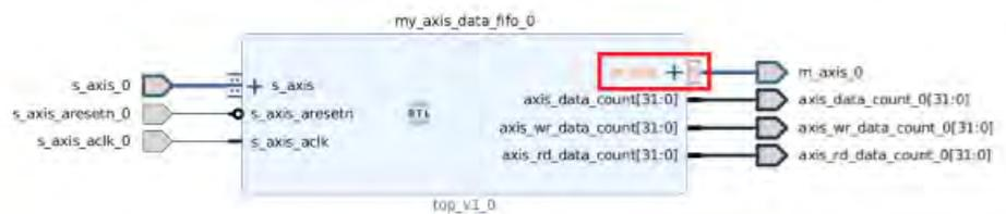
To auto associate the **s\_axis\_aclk** to both the **s\_axis** and the **m\_axis** interfaces, rename the clock in your RTL code to **axis\_aclk**.
