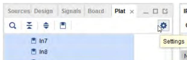
Clicking the Settings button brings up the menu to select or de-select the desired interfaces. The grayed out interfaces are interfaces that are not available in the particular platform.
