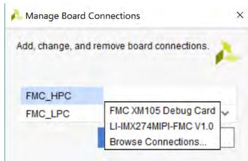
As shown, when KC705 is selected, the FMC\_HPC and FMC\_LPC connectors show the available FMC cards. Selecting a card enables all the connections on that card available for use in the design.
