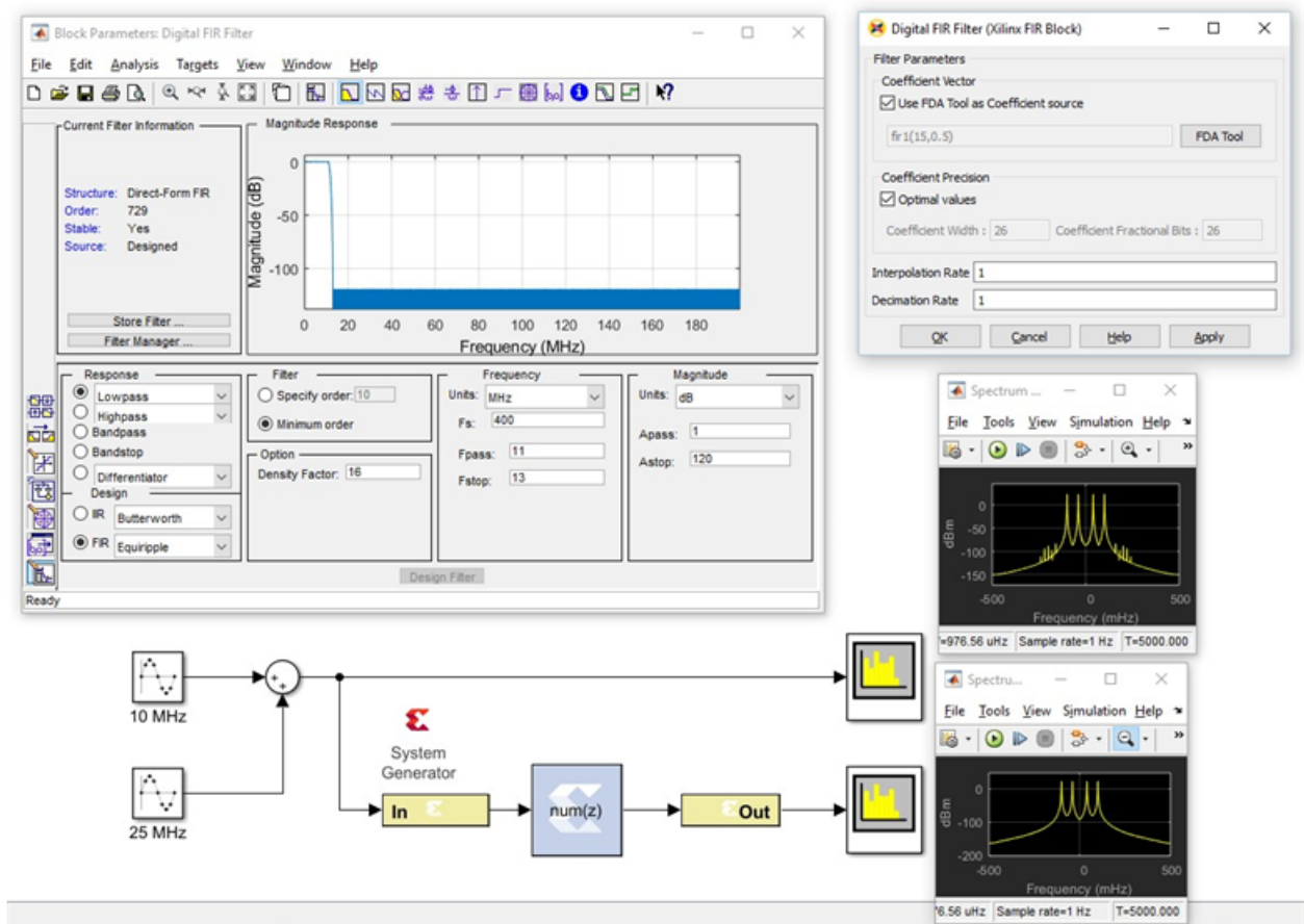
Figure 20: Digital FIR Filter Example
