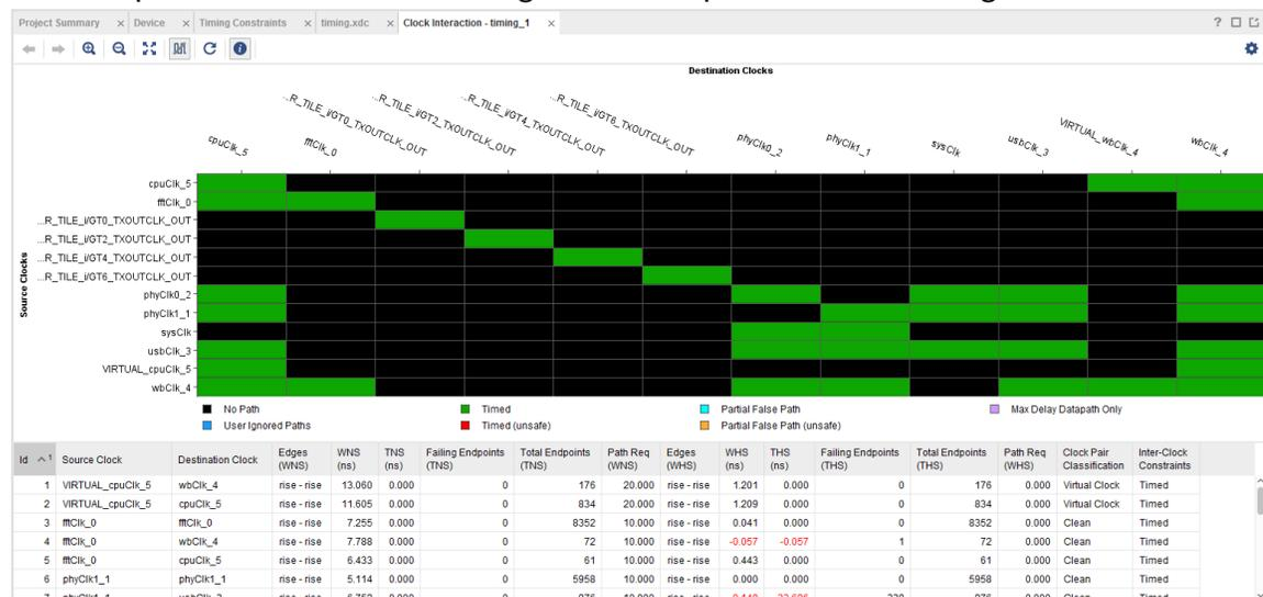
The Vivado IDE generates a graphical matrix illustrating the relationship of the various clocks in the design, as shown in the previous figure. For this design, the primary clock (`sysCk`) connects to an MMCM, which generates six additional clocks. The clock interactions shown are between these generated clocks. In addition, the Timing Constraints wizard created additional generated clocks and virtual clocks to fully constrain the design.
