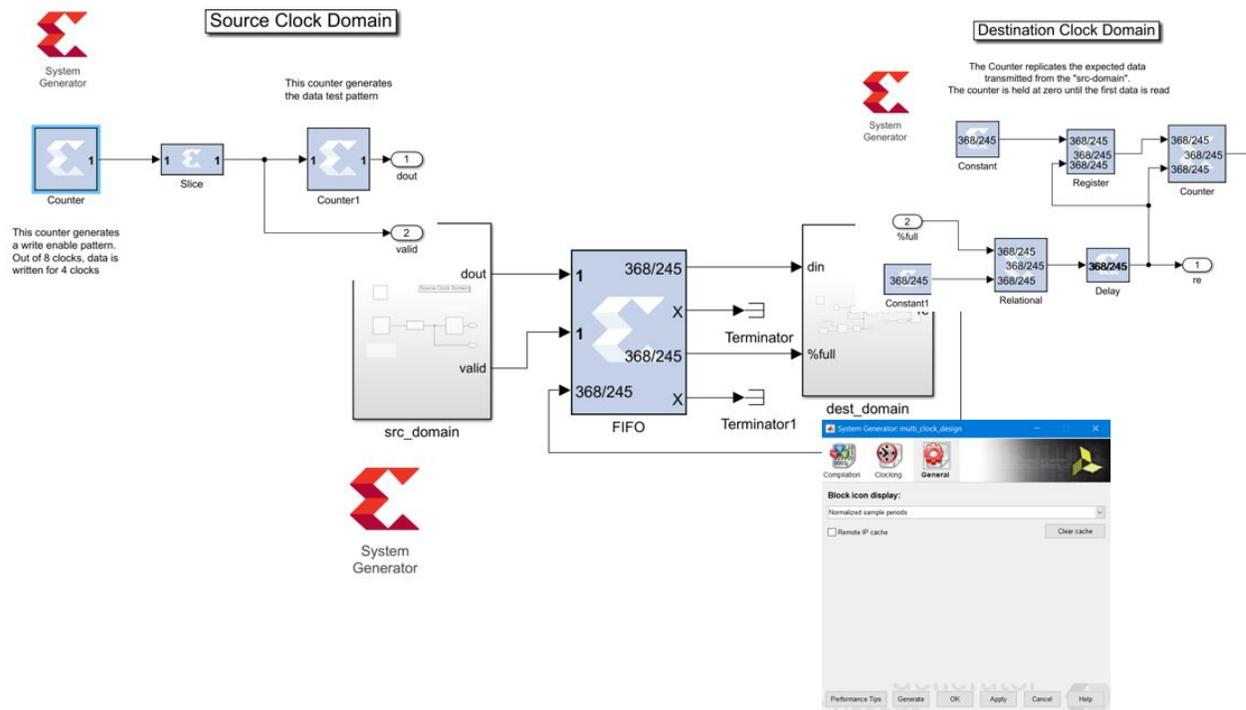
To enable the above display, set the **Block icon display** of the top-level System Generator token to **Normalized Sample Periods** and press **Apply**.
