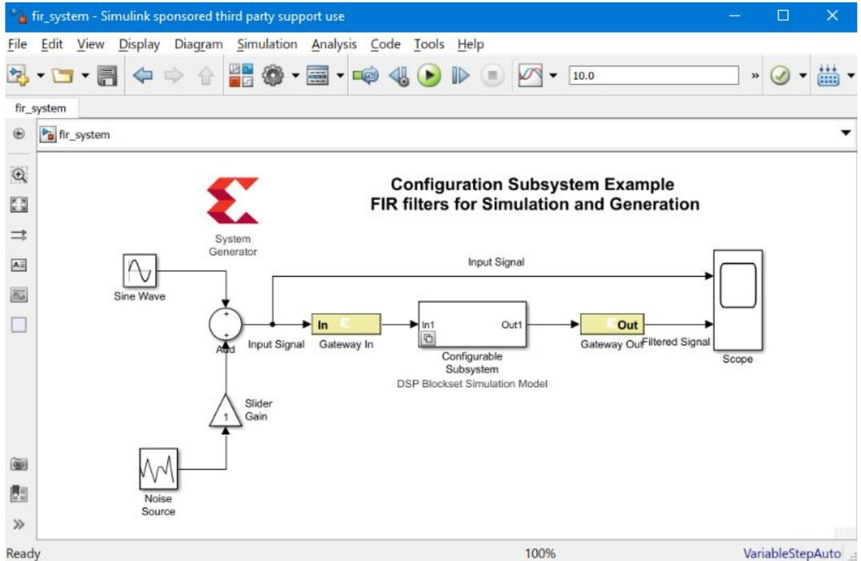
5. Right-click the instance, and under **Block Choice** select the block that should be used as the underlying implementation for the instance.
