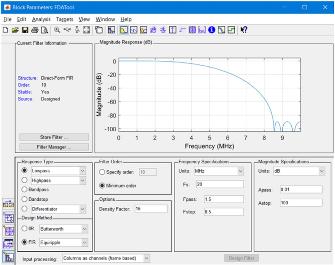
The Design Filter option at the bottom of the tool window allows you to find out the filter order and observe the Magnitude Response. You can also view the Phase Response, Impulse Response, Coefficients, and more by selecting the appropriate icon at the top-right of the window. You can display the filter coefficients in the MATLAB® workspace by typing the following:
