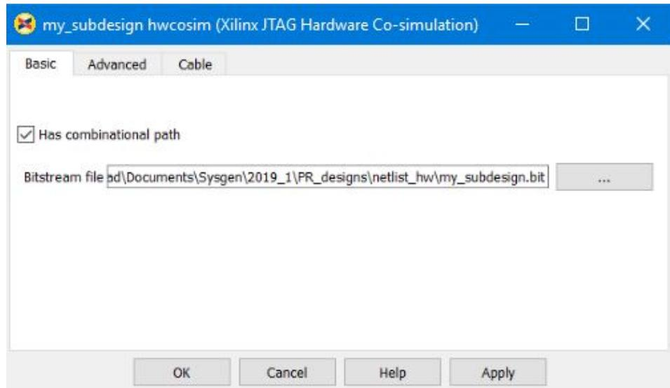
3. Fill out the block parameters in the properties dialog box.
