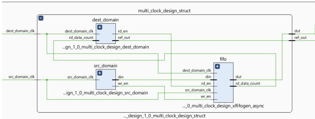
As many clock ports as there are clock domains are exposed at the top level and can be driven by a variety of Xilinx clocking constructs like MMCM, PLL etc. It is assumed that these clocks are completely asynchronous and the following period constraints are created:
