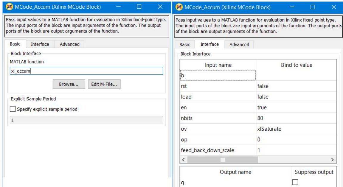
The example contains two additional accumulator Subsystems with MCode blocks using the same M-function, but different parameter settings to accomplish different accumulator implementations.
