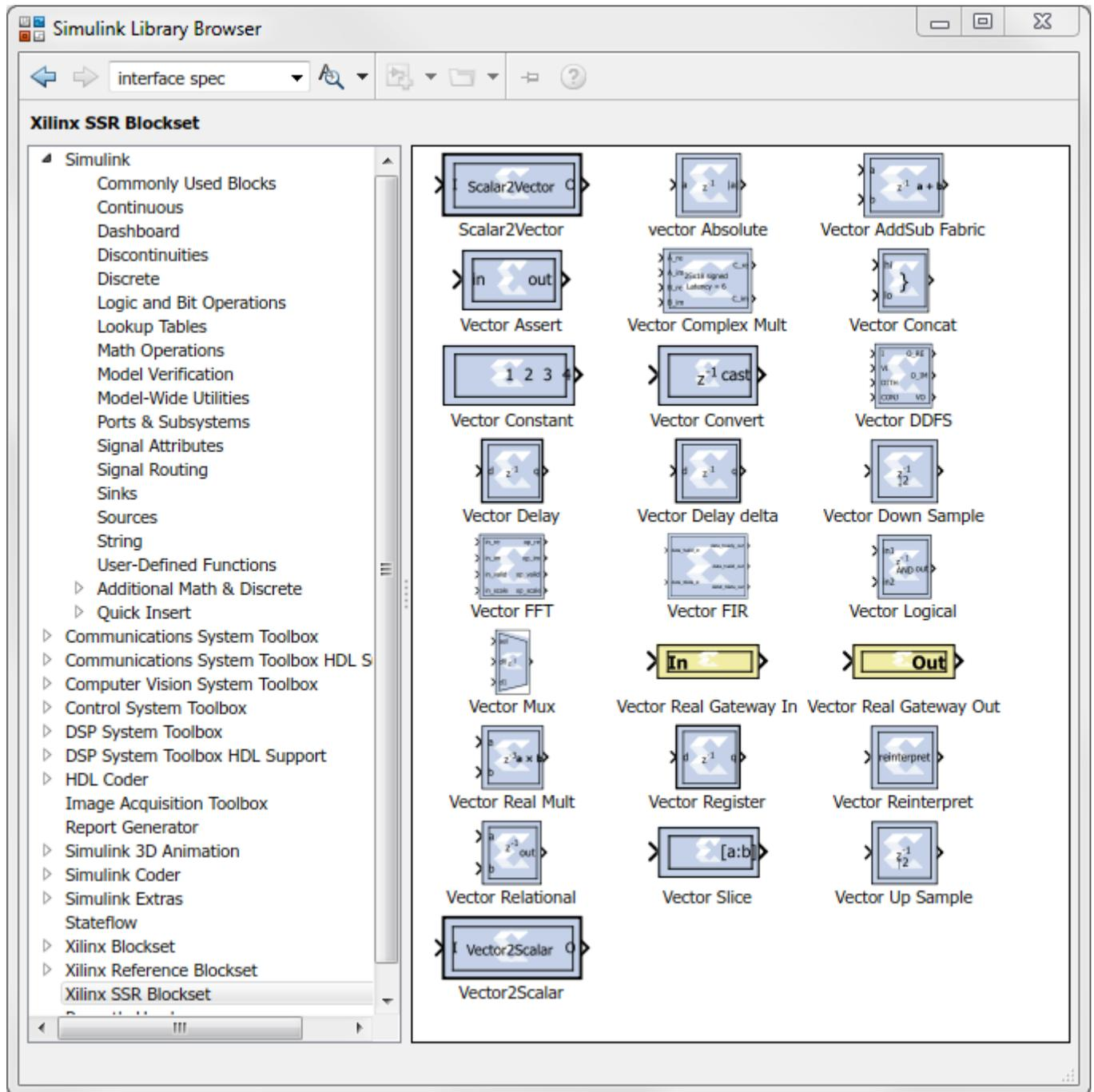
The SSR parameter can be defined for all the blocks present in the SSR block set. When you add a block from the library, the default SSR value is 4, and the maximum SSR value is 256.
