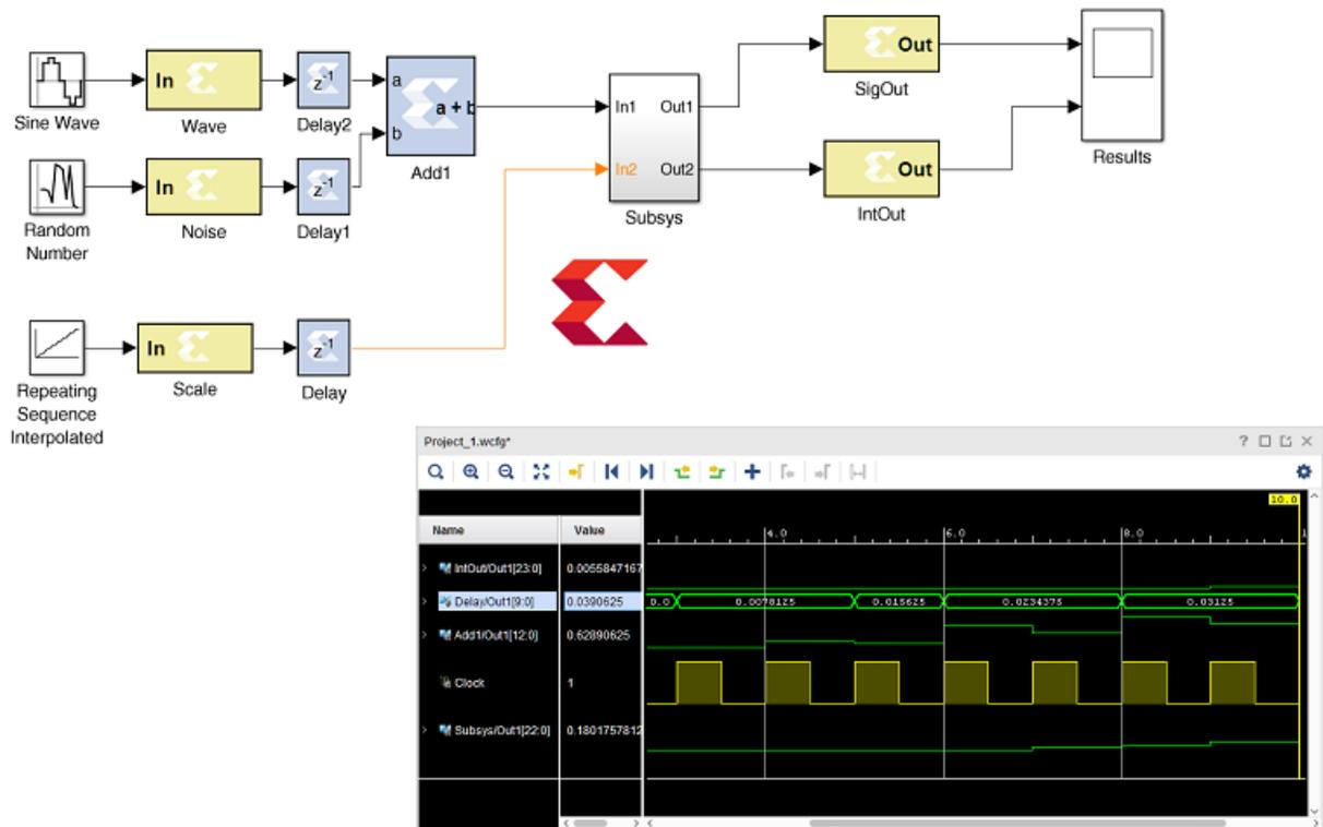
The Xilinx Waveform Viewer used with System Generator is also used by other tools in the Vivado® toolset. The Waveform Viewer is used to analyze a design and debug code in the Vivado simulator and to display data captured by the Integrated Logic Analyzer (ILA) for in-system debugging.
