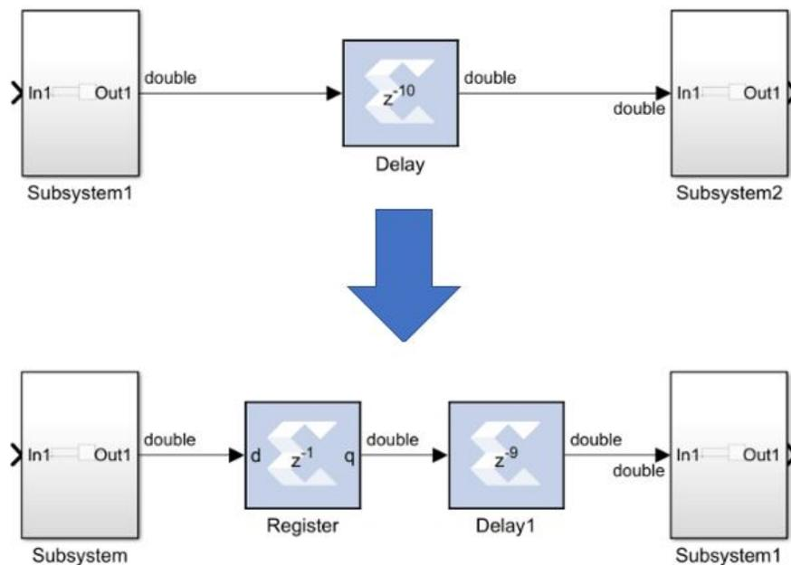
As shown in the following figure, the Convert block can be pipelined with embedded register stages to guarantee maximum performance.
