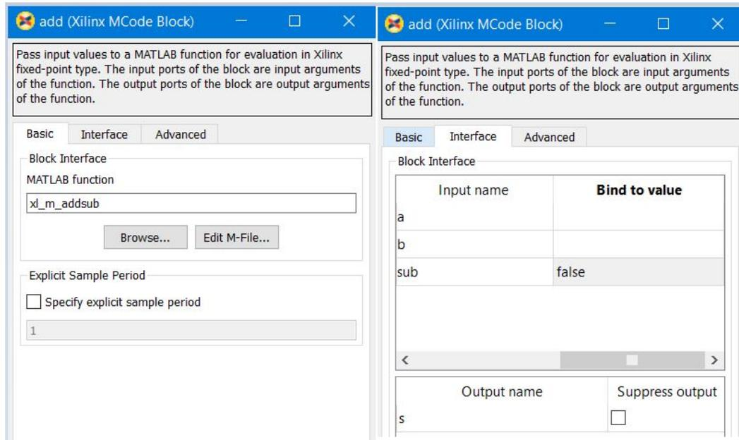
As a result, the `add` block features two input ports `a` and `b`; it performs full precision addition. Input parameter `sub` of the MCode block labeled `addsub` is not bound with any value. Consequently, the `addsub` block features three input ports: `a`, `b`, and `sub`; it performs full precision addition or subtraction based on the value of input port `sub`.
