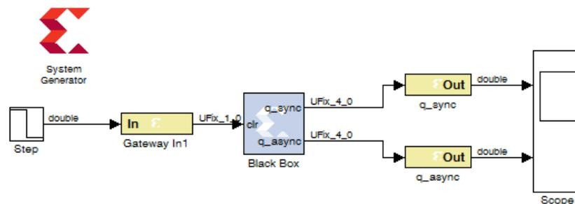
The next step is to double-click the System Generator token and click the **Generate** button to generate the HDL netlist.
