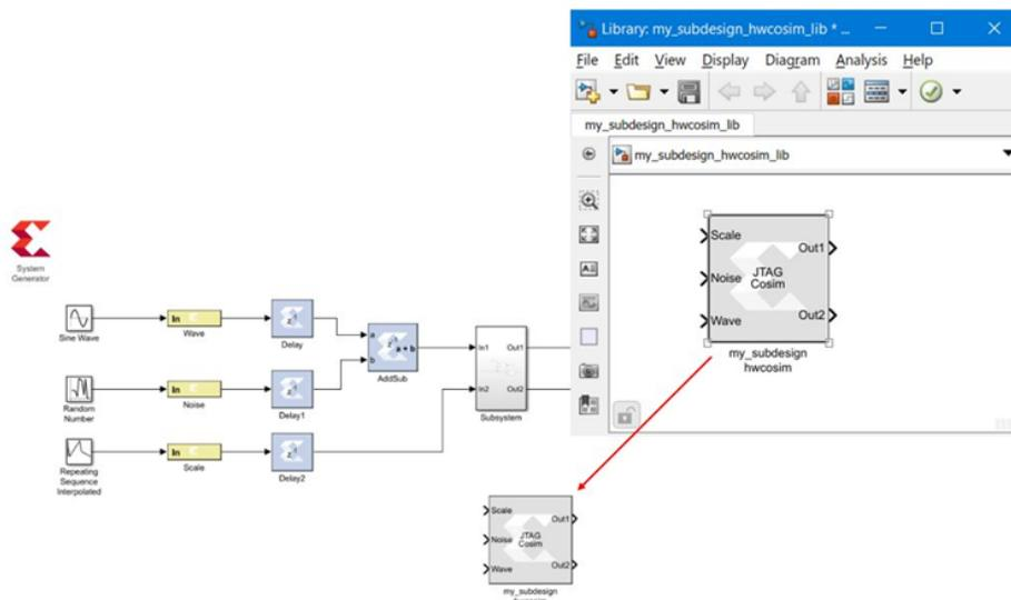
If you selected the **Create Testbench** option for compilation, an M-Code HWCosim example test bench will also be generated (see [M-Code Access to Hardware Co-Simulation](#)) by the compilation. You can use this test bench to perform hardware co-simulation, or customize this test bench to develop a test bench of your own.
