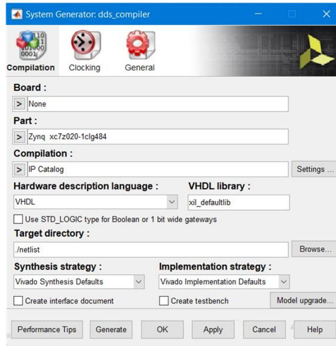
The System Generator block must first be configured to a Compilation target of **IP Catalog** (the default generation target). This compilation target will consolidate all hardware source created from System Generator (RTL + IP + Constraints) into an IP.
