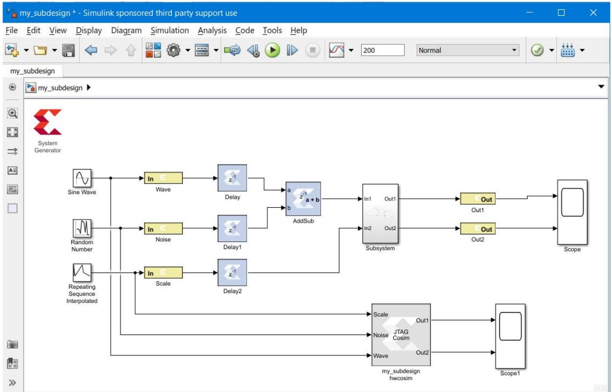
2. Double-click the hardware co-simulation block to display the properties dialog box for the block.
