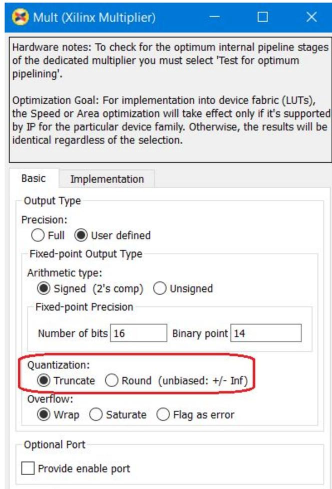
In order to use a parameter rather than the radio button selection, right-click the radio button and select **Define With Expression**. A MATLAB expression can then be used as the parameter setting. In the example below, the `trunc_round` parameter from the Subsystem mask can be used in both the accumulator and multiply blocks so that each block will use the same setting from the mask variable on the Subsystem.
