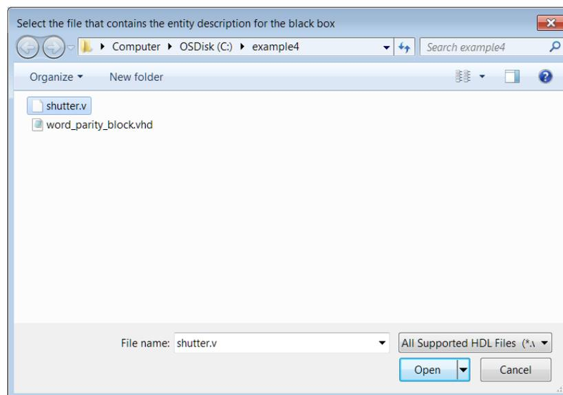
You can select the file you would like to import by selecting the file, and then pressing the **Open** button. At this point, the configuration wizard generates a configuration M-function, and associates it with the black box block.
