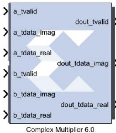
The breaking out of multi-channel TDATA does not add additional logic to the design and is done in System Generator as a convenience to the users. The data in each broken out TDATA port is also correctly byte-aligned.
