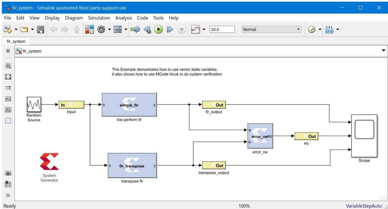
The model contains two FIR blocks. Both are modeled with the MCode block and both are synthesizable. The following are the two functions that model those two blocks.
