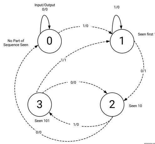
The M-function that is used by the MCode block contains a transition function, which computes the next state based on the current state and the current input. Unlike example 3 though, the M-function in this example defines persistent state variables to store the state of the finite state machine in the MCode block. The following M-code, which defines function
