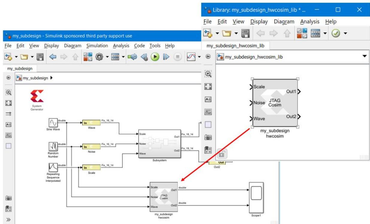
The hardware co-simulation block assumes the external interface of the model or Subsystem from which it is derived. The port names on the hardware co-simulation block match the ports names on the original Subsystem. The port types and rates also match the original design.
