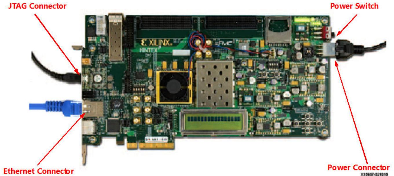
To set up the KC705 board for Point-to-Point Ethernet hardware co-simulation:
