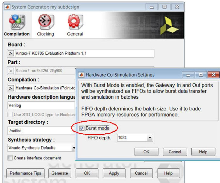
Enabling **Burst mode** allows the M-HWCosim scheduler to "burst write" a time-sequence of "n" values into each input FIFO, run the clock for a number of cycles determined by the rate of input/output ports and the FIFO depths, and capture the resulting output in the output FIFOs. After the batch has been run, the scheduler proceeds to "burst read" the contents of the output FIFOs into a MATLAB array, where it can be checked against expected data.
