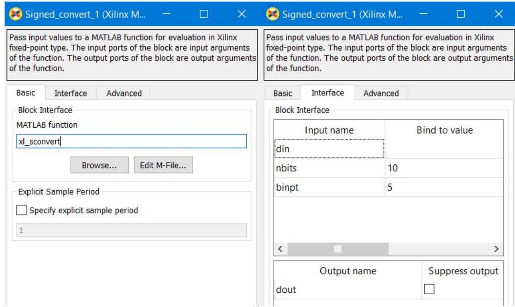
The above interface window sets the M-function argument `nbits` to be 10 and `binpt` to be 5. The mask for the MCode block `signed_convert_2` is shown below:
