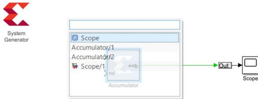
If a second connection is made to this Scope block, a second port is automatically added to the Scope. The driving signal name is also used to name the signal driving the scope.
