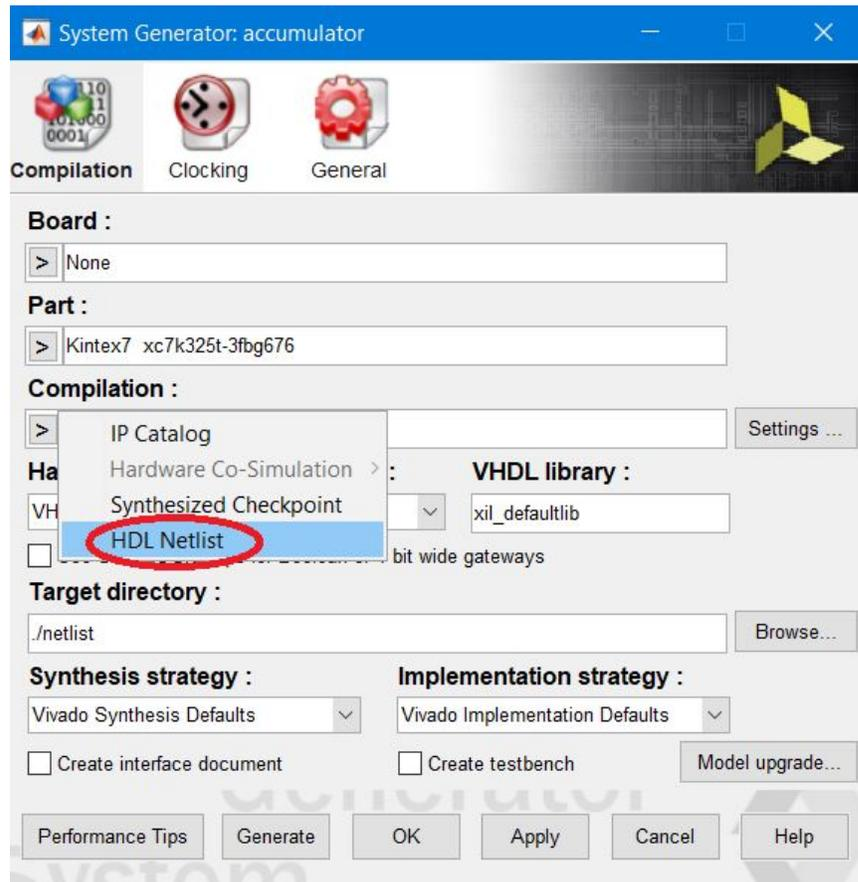
The **Board** and **Part** fields allow you to specify the board or part for which you are targeting the **HDL Netlist** compilation. When you select a **Board**, the **Part** field automatically displays the name of the Xilinx® device on the selected **Board**, and this part name cannot be changed.
