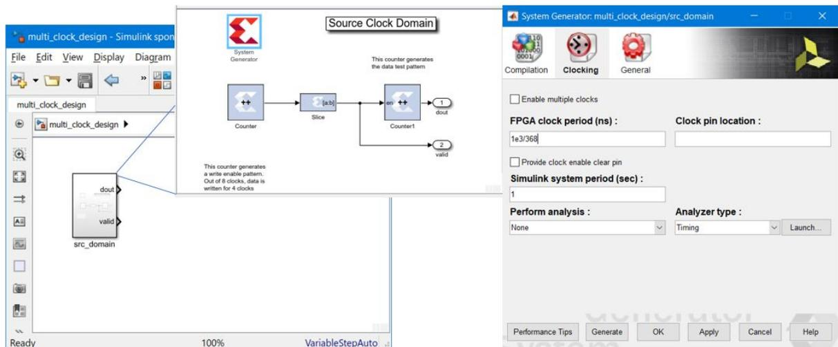
In this figure, a clock domain Subsystem called `src_domain` has been created and a System Generator token added. Notice that the clocking tab of the System Generator token is selected. In this tab, the FPGA clock period has been set to (1000/368) ns (368 MHz) and the Simulink system period to 1. This implies that an advance of 1 Simulink second corresponds to (1000/368) ns of FPGA clock.
