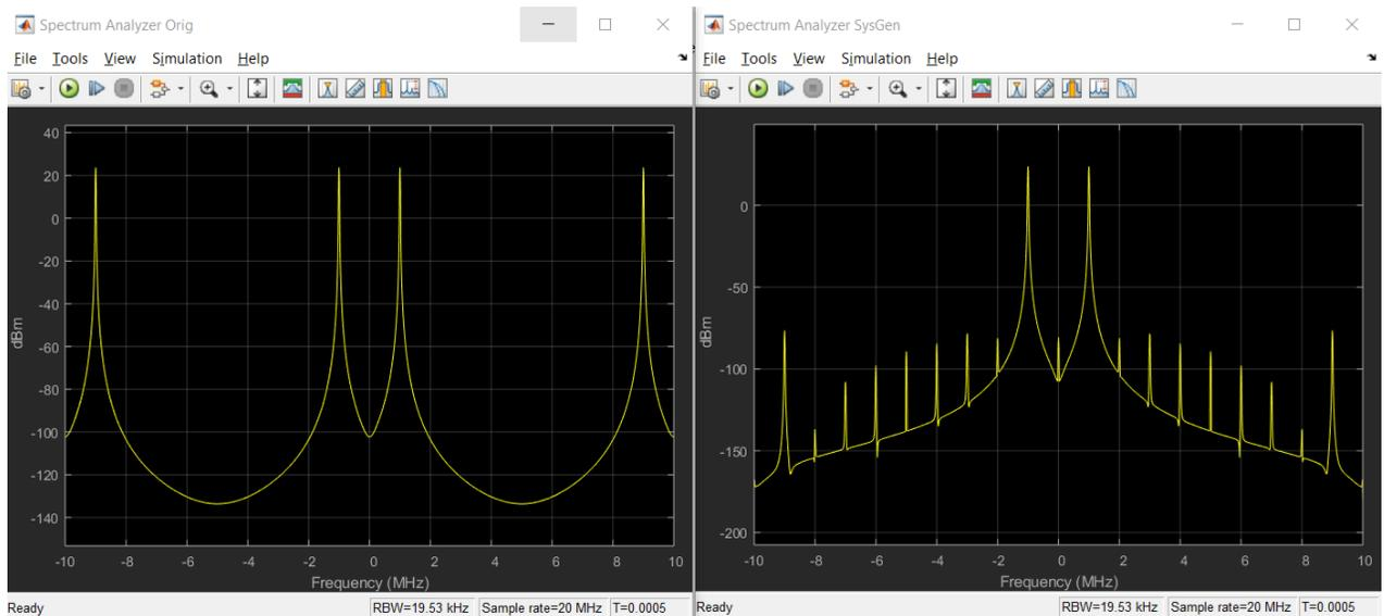
**Note:** The frequency response results of System Generator (right side), shown above, differs slightly with the original design (left side) due to the quantization and sampling effect inherent when a continuous time system is described in discrete time hardware.
