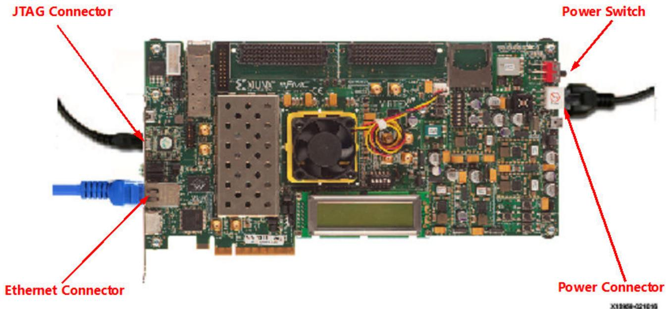
To set up the VC707 board for Point-to-Point Ethernet hardware co-simulation:
