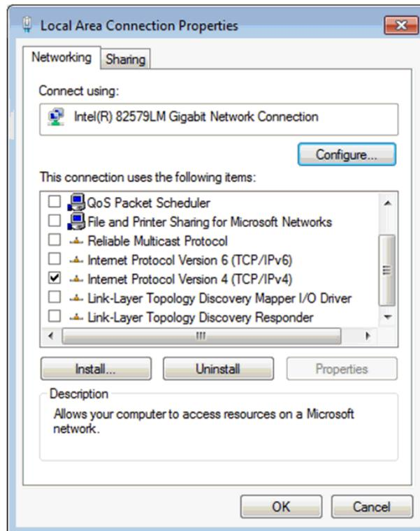
4. Select **Internet Protocol Version 4 (TCP/IPv4)**, and click **Properties**. In the Internet Protocol Version 4 (TCP/IPv4) dialog box, select **Use the following IP address**, and set the **IP Address** to 192.168.1.11, and **Subnet mask** to 255.255.255.0. Click **OK**.
