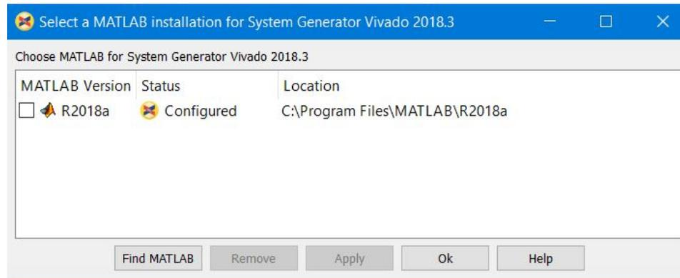
This dialog box allows you to associate any supported MATLAB® installation with this version of System Generator.
