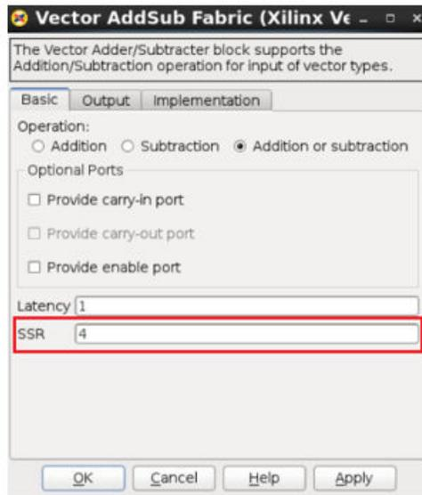
No matter what the SSR rate is, you only need to provide a limited number of signal connections as with a normal IP block. System Generator automatically takes care of all the parallel path connection internal to the SSR block, according to the SSR parameter value provided.
