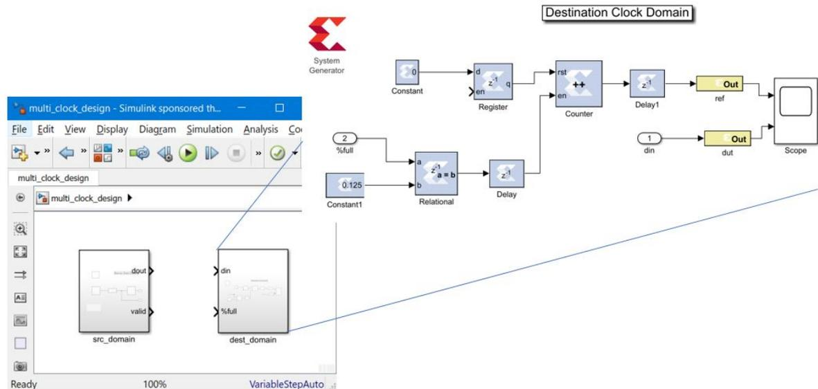
In this design, the `dest_domain` Subsystem is configured to run at an FPGA clock period of  $1000/245$  ns (245 MHz). The Simulink system period is set to  $368/245$ . This is done because the Simulink system period of the `src_domain` Subsystem is set to 1. Hence, you normalize with the System period from the `src_domain` which is faster.
