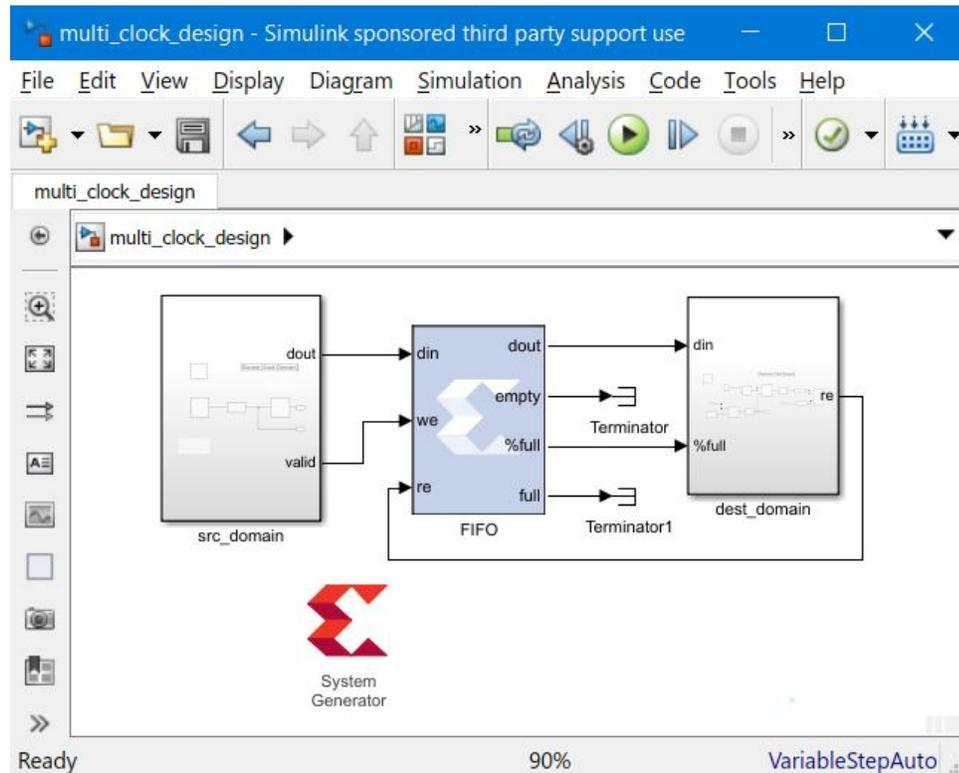
To complete the design, the FIFO block and an additional System Generator block at the top level of the design is included to enable Code Generation.
