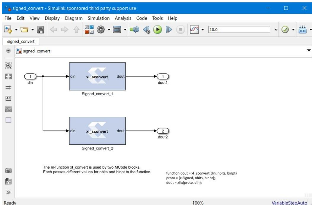
To pass parameters to each MCode block in the diagram above, you can click the **Edit M-File** button on the block GUI then set the values for the M-function arguments. The mask for MCode block `signed convert 1` is shown below:
