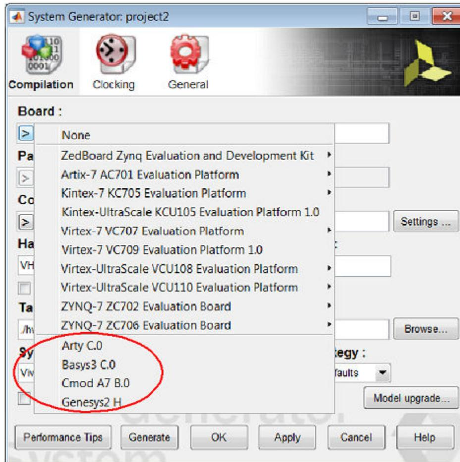
To add an additional board to your board repository, you can modify the `xilinx.environment.setBoardFileRepos` line in your `startup.m` file to point to the location of the new Board Interface file (`board.xml`). If you place the Board Interface file in a subdirectory under a folder already specified in the `xilinx.environment.setBoardFileRepos` line, the new board will be available the next time you open System Generator, without having to make any changes to the `startup.m` file.
