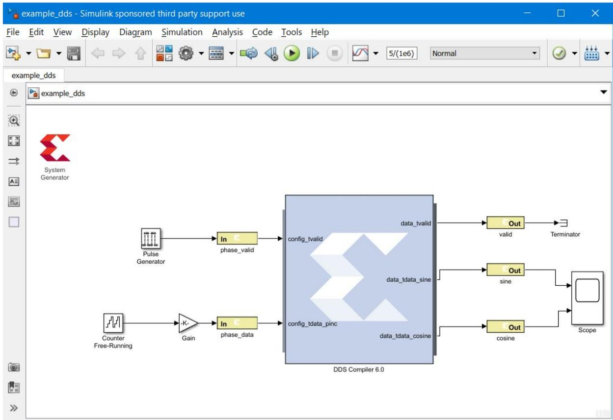
This design contains a DDS Compiler where the two input ports, `config_tvalid` and `config_tdata_pinc` are used to control the output frequency.
