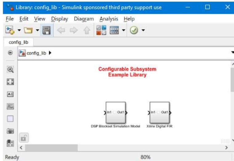
3. Drag a template block into the library. (Templates can be found in the Simulink library browser under Simulink/Ports & Subsystems/Configurable Subsystem.)
