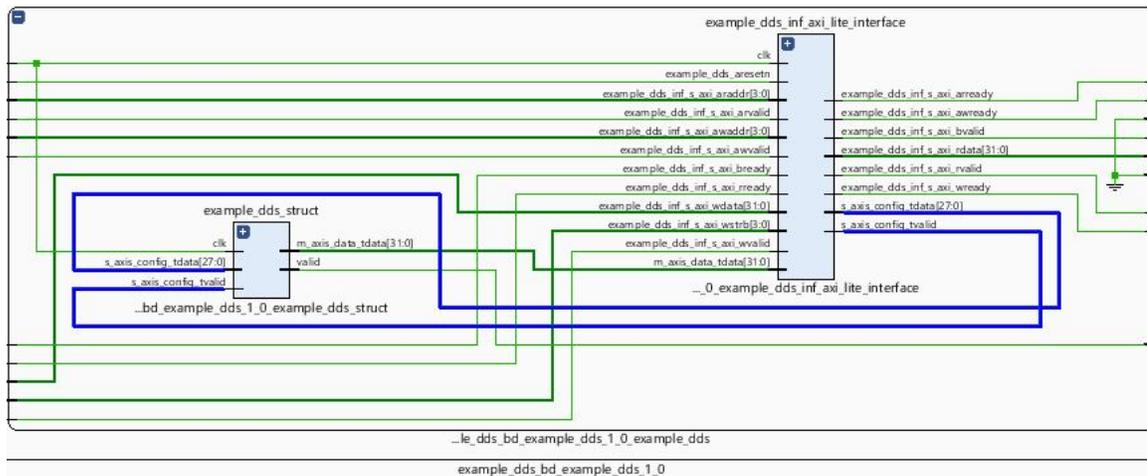
As you can see in the diagram, a module called `example_dds_inf_axi_lite_interface` is inserted into the design RTL, and drives the `config_tvalid` and `config_tdata` ports of the System Generator design. And at the top level, a slave AXI4-Lite Interface is exposed. It is within this module that address decoding is done and the `config_tvalid` and `config_tdata` ports are driven based on the address obtained from the processor.
