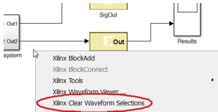
To open the Waveform Viewer again, right-click in your model and select **Xilinx Waveform Viewer** in the right-click menu. The Waveform Viewer opens displaying waveforms for the clock signals in your design, and no other waveforms.
