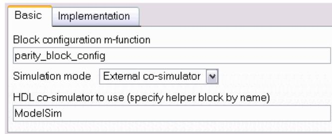
Configuration M-functions use an object-based interface to specify black box information. This interface defines two objects, `SysgenBlockDescriptor` and `SysgenPortDescriptor`. When System Generator invokes a configuration M-function, it passes the function a block descriptor:
