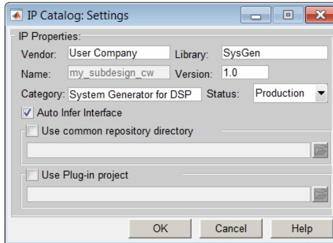
The **Use common repository directory** field allows you to specify a directory referred to as the Common Repository. In an IP catalog compilation, the IP created is copied over to this location. If a Vivado user adds this Path as User Repository in the Vivado project's IP Settings, then all IPs that a System Generator user has placed in this Common Repository will automatically be picked up by Vivado and can be used either in an IP integrator or an RTL flow.
