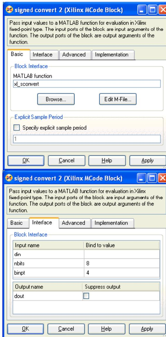
The above interface window sets the M-function argument `nbits` to be 8 and `binpt` to be 4.
