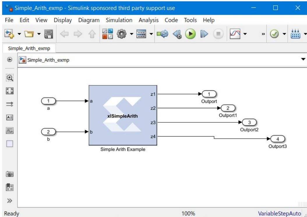
M-functions using Xilinx data types and functions can be tested in the MATLAB Command Window. For example, if you type: `[z1, z2, z3, z4] = xlSimpleArith(2, 3)` in the MATLAB Command Window, you'll get the following lines:
