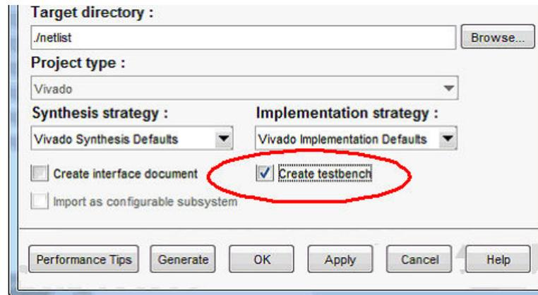
As shown below, when you include a test bench, you can verify the IP functionality by adding three more steps to the flow.
