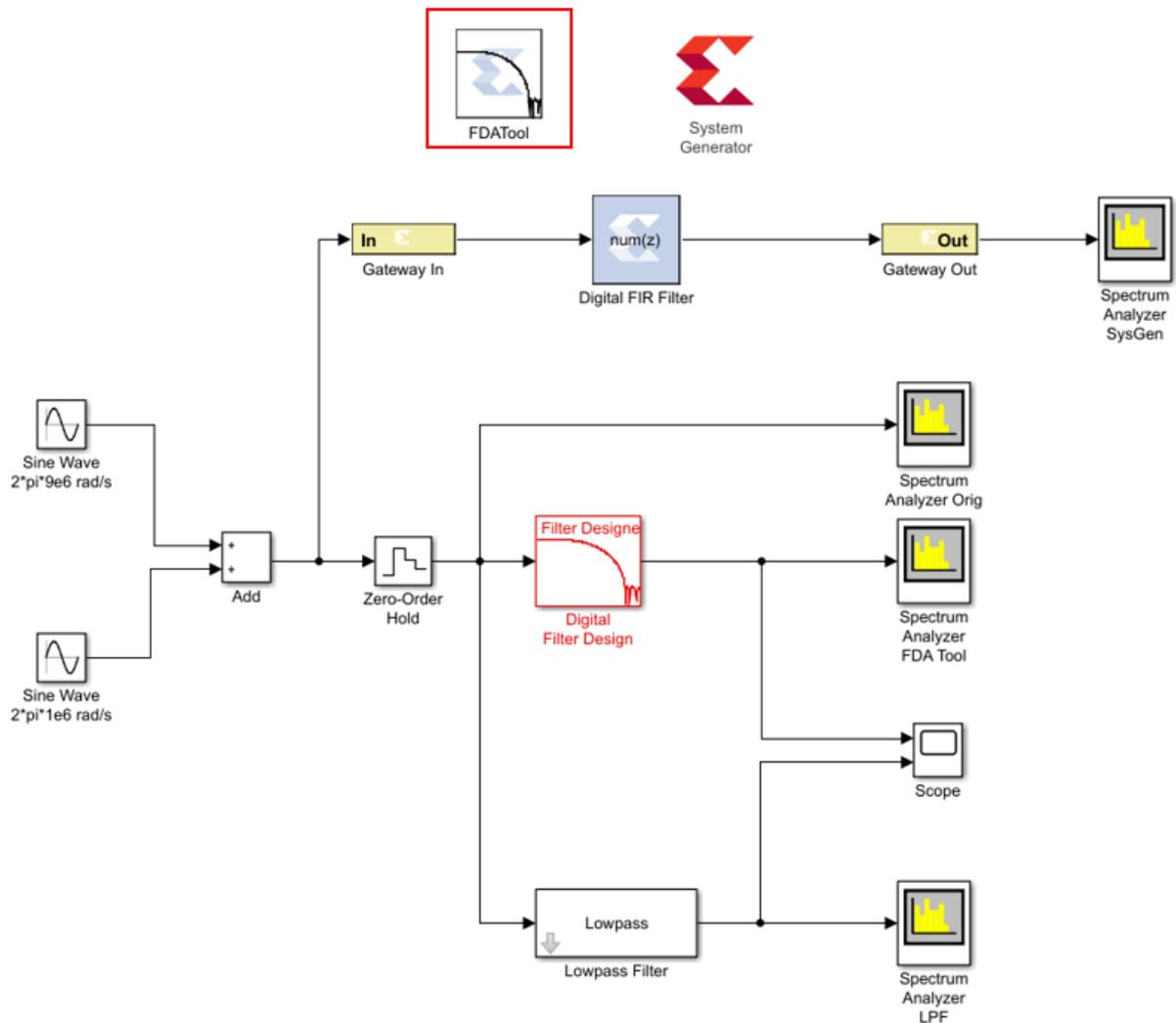
The Xilinx version of the FDAtool can be used to define the coefficients of the low-pass filter to eliminate high-frequency noise. The filter configuration parameters like Response Type, Filter Order, Frequency Specification, and Magnitude Specification can be modified from the Properties Editor of the FDAtool as shown below.
