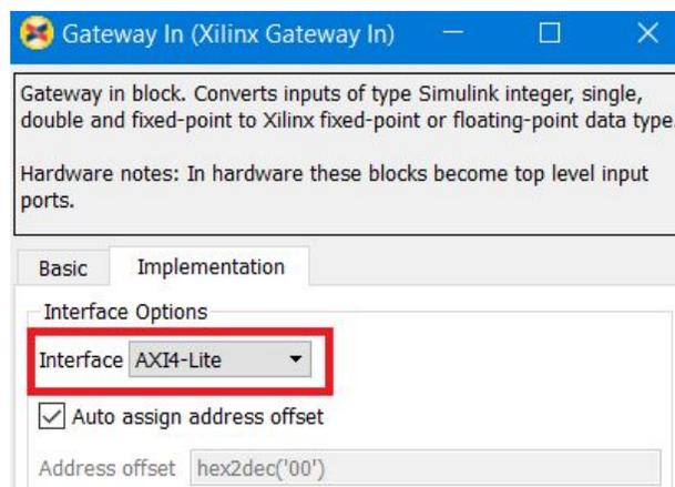
As you can see, the Interface is specified as a slave AXI4-Lite Interface in System Generator, which means that it will be transformed to a top-level AXI4-Lite interface.
