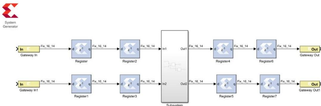
Double registering the I/Os may also be beneficial. This can be performed by instantiating two separate Register blocks, or by instantiating two Delay blocks, each having latency 1. This allows one of the registers to be packed into the IOB and the other to be placed next to the logic in the FPGA fabric. A Delay block with latency 2 does not give the same result because the block with a latency of 2 is implemented using an SRL32 and cannot be packed into an IOB.
