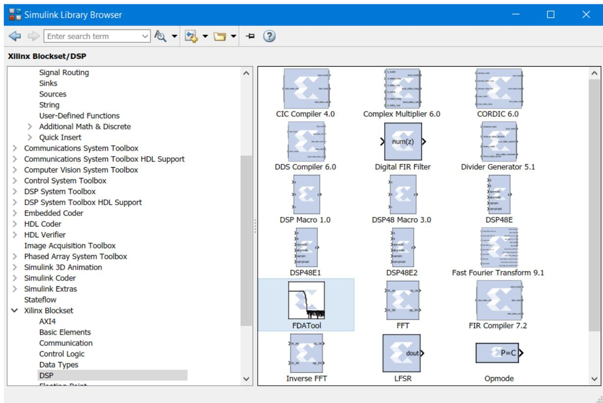
A simple System Generator model below illustrates a standard FIR filter design using the FDATool and digital FIR filter block.
