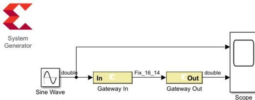
The Gateway In block is configured with a sample period of one second. The Gateway Out block converts the Xilinx fixed-point signal back to a double (so it can be analyzed in the Simulink scope), but does not alter sample rates. The scope output below shows the unaltered and sampled versions of the sine wave.
