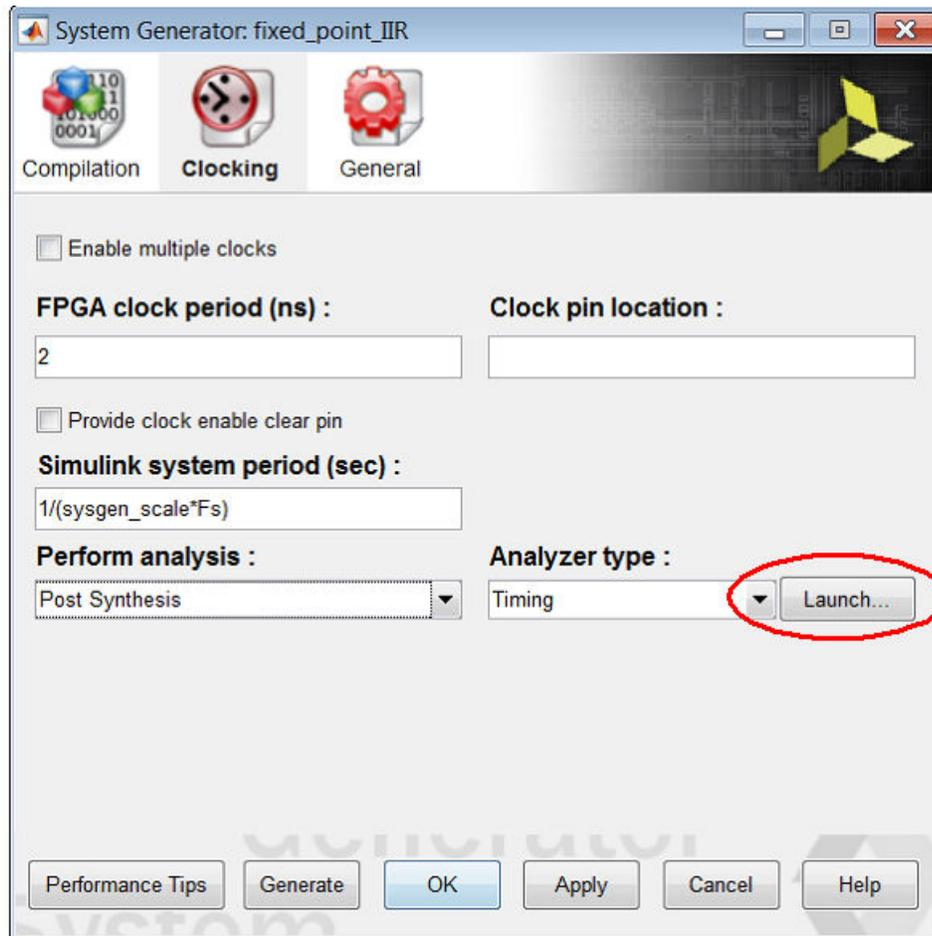
You can also launch the Timing Analyzer table to display existing timing analysis results by entering this command at the MATLAB® command prompt:
