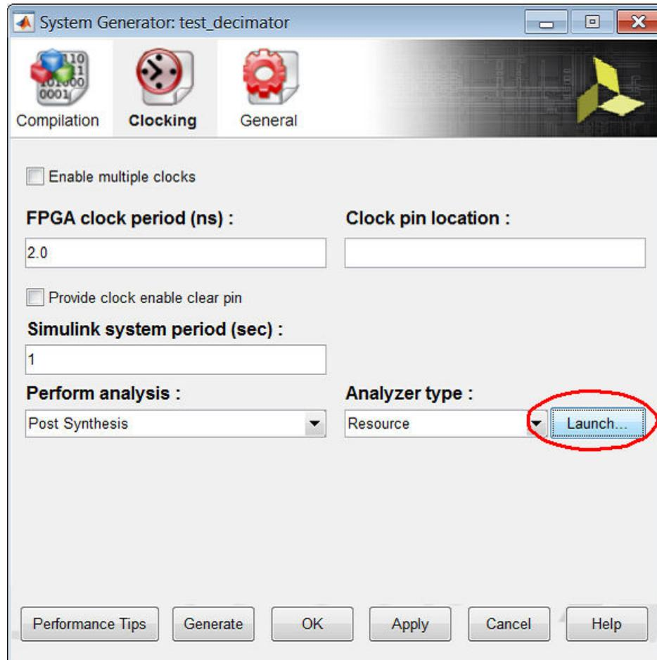
You can launch the Resource Analyzer table to display existing resource utilization results by entering the following command at the MATLAB® command prompt:
