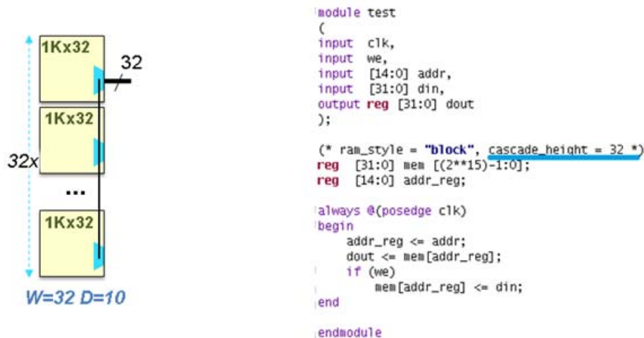
Figure 3-23: RTL Representation of 32Kx32 Using 1Kx32 and CASCADE_HEIGHT=32
