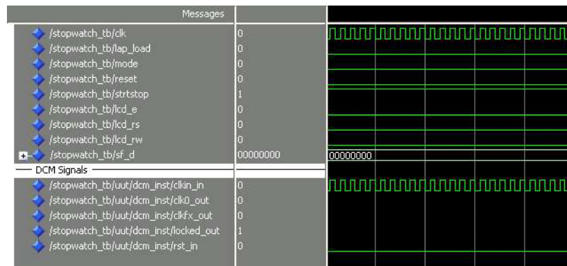
Figure 5-6: Waveform After Adding DCM Signals Divider
