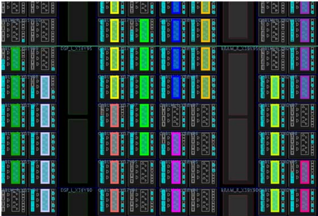
Figure 5-25: DSP48 Implemented in CLBs
