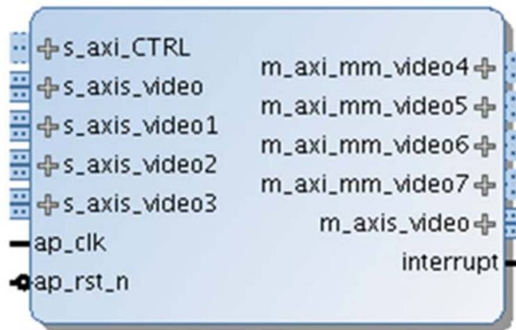
Figure 2-1: Video Mixer I/O Diagram
