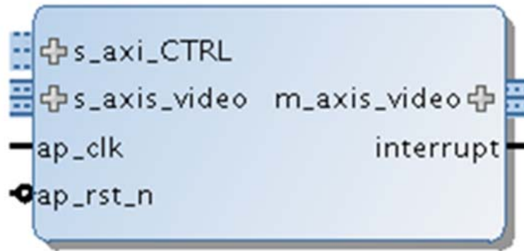
Figure 2-2: Video Mixer I/O Diagram Single Layer
