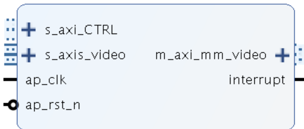
Figure 2-2: Video Frame Buffer Write I/O Diagram
