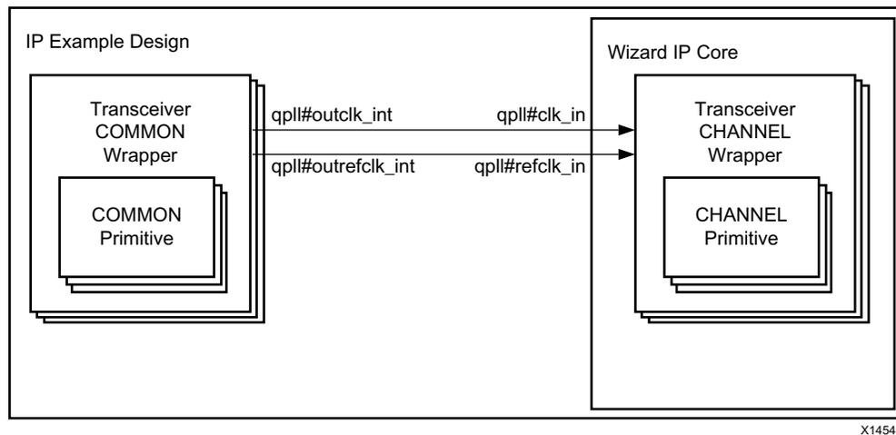
Figure 3-9: Transceiver Common Located in the Example Design
