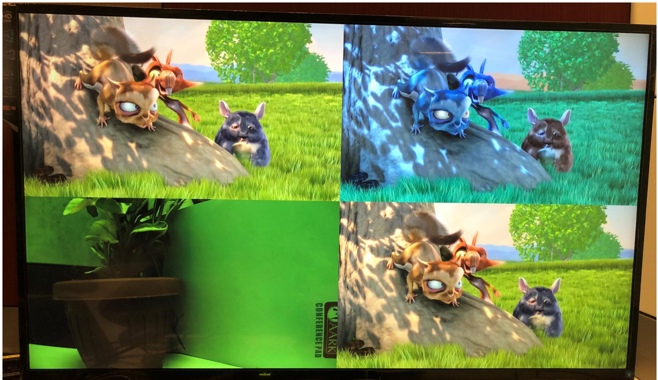
Figure 3-18: Multi-Stream—3 HDMI and 1 MIPI Input Sources @ 1080p60
