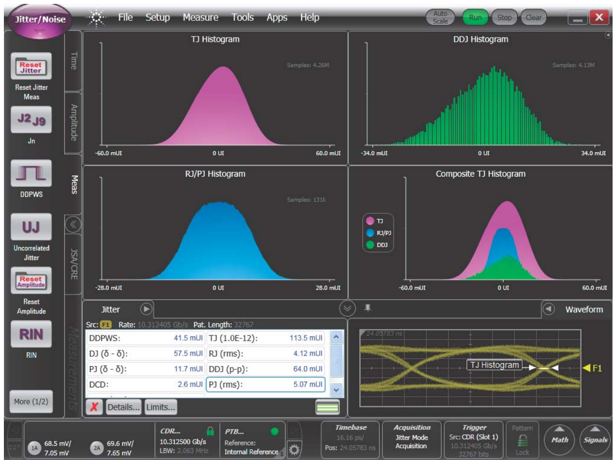
Figure 11: 10.3125 Gb/s Output Jitter Decomposition
