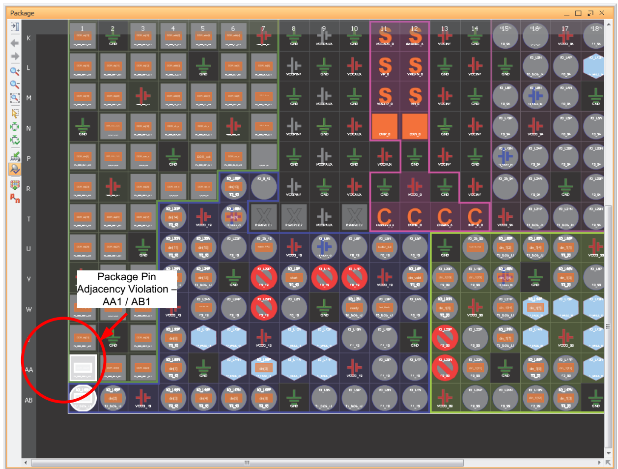
Figure 30: Package Pin Adjacency Violation - Package View
