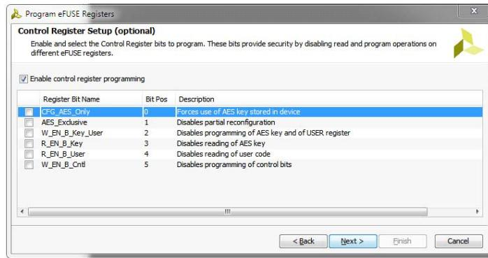
Figure 4: eFUSE Programming GUI (Control Register Setup)
