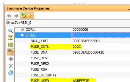
Figure 5: Hardware Device Properties/EFUSE Register Drop-Down Menu
