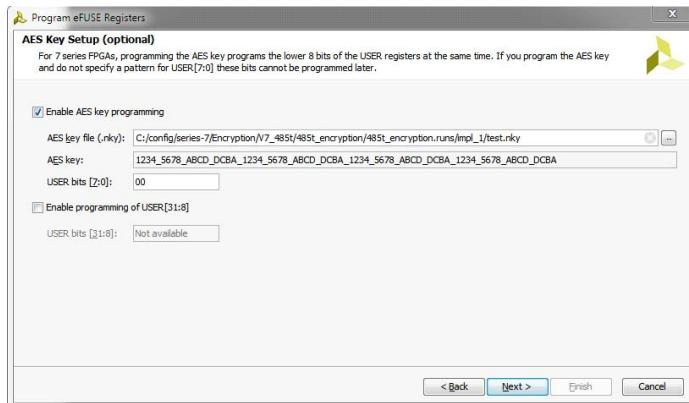
*Figure 3: eFUSE Programming GUI (AES Key Setup)*
