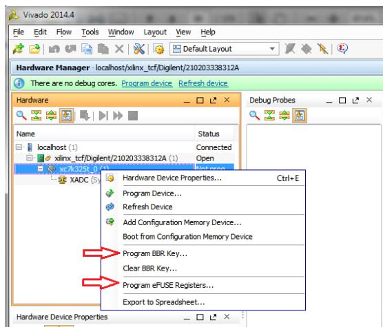
[Figure 1: Vivado Tools HW Manager Key Programming Selection](#)
